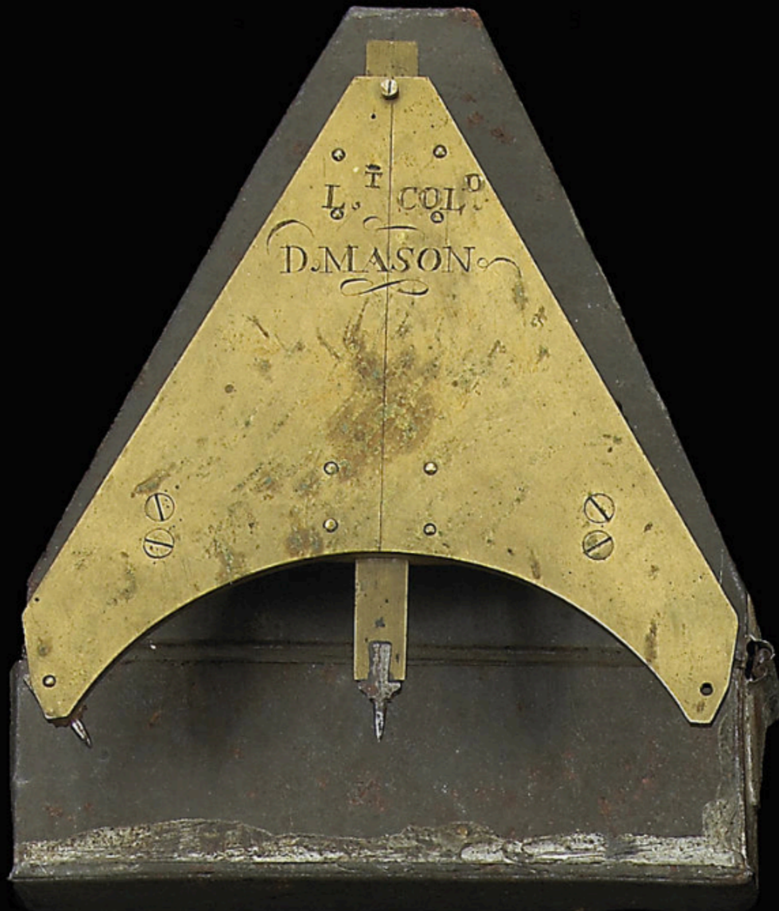
Cased Gunner's Perpendicular Owned by Lt. Colonel David Mason of Boston c. 1777
