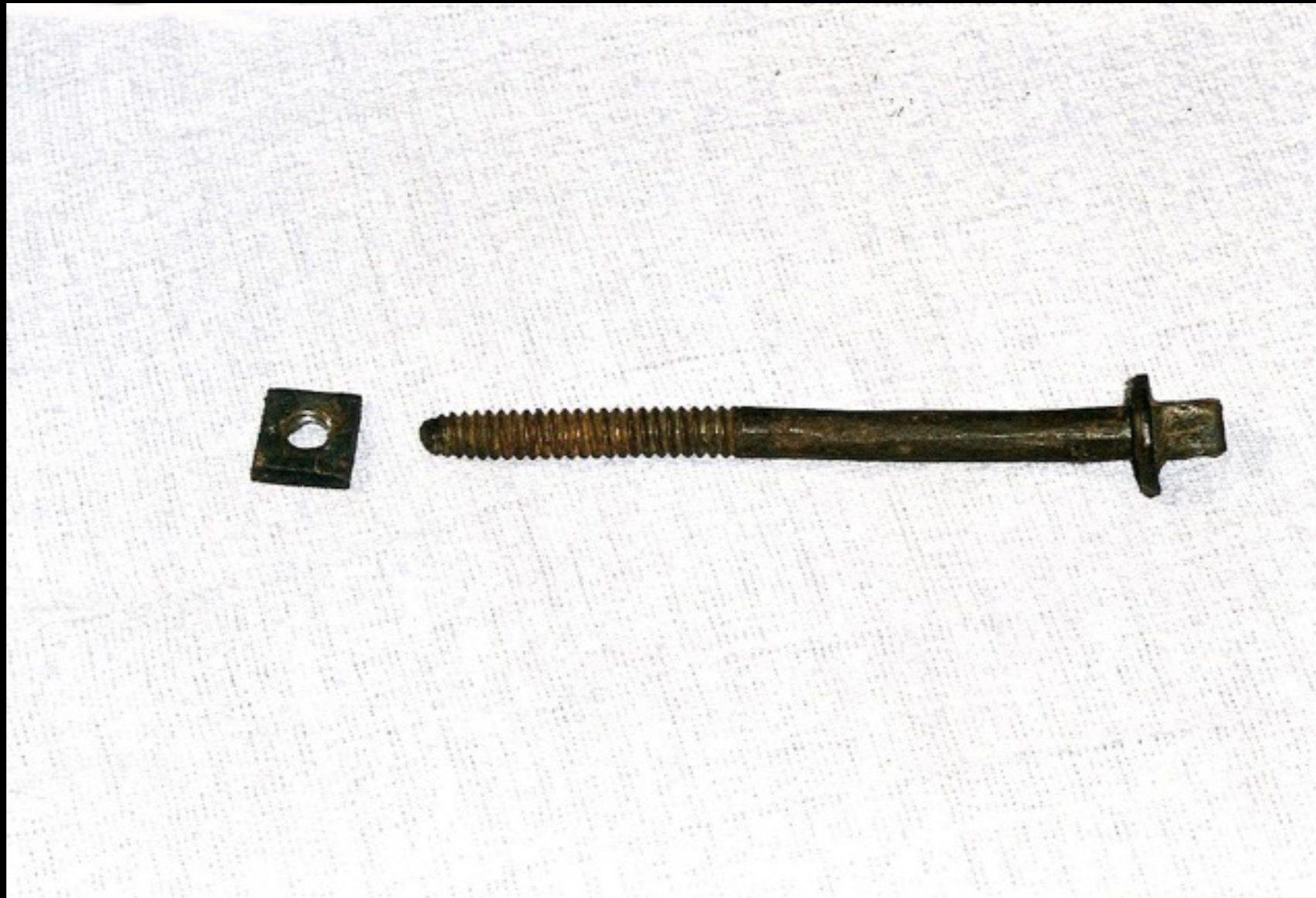
Handmade Iron Bed Bolt with Nut Used to Assemble a Bed The Nut Was Implanted in the Rail and the Bolt was Tightened by an Iron Bed Wrench Often the Assembly was Hidden by a Decorative Cover 18th Century (Fred Taylor, Auction Central News)
