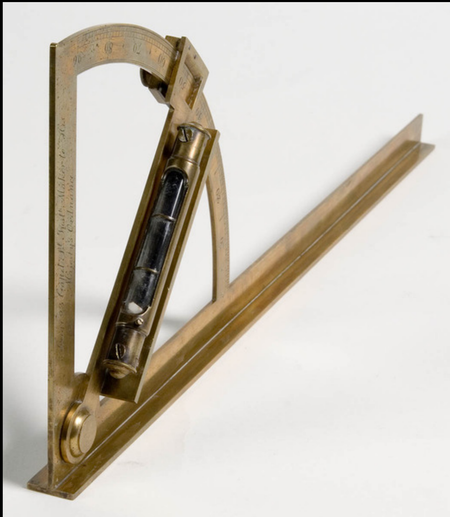
Inclinometer, or Gunner's Quadrant, Used for Leveling in Shore Work - Associated with Captain James Cook 18th Century (State Library - New South Wales)
