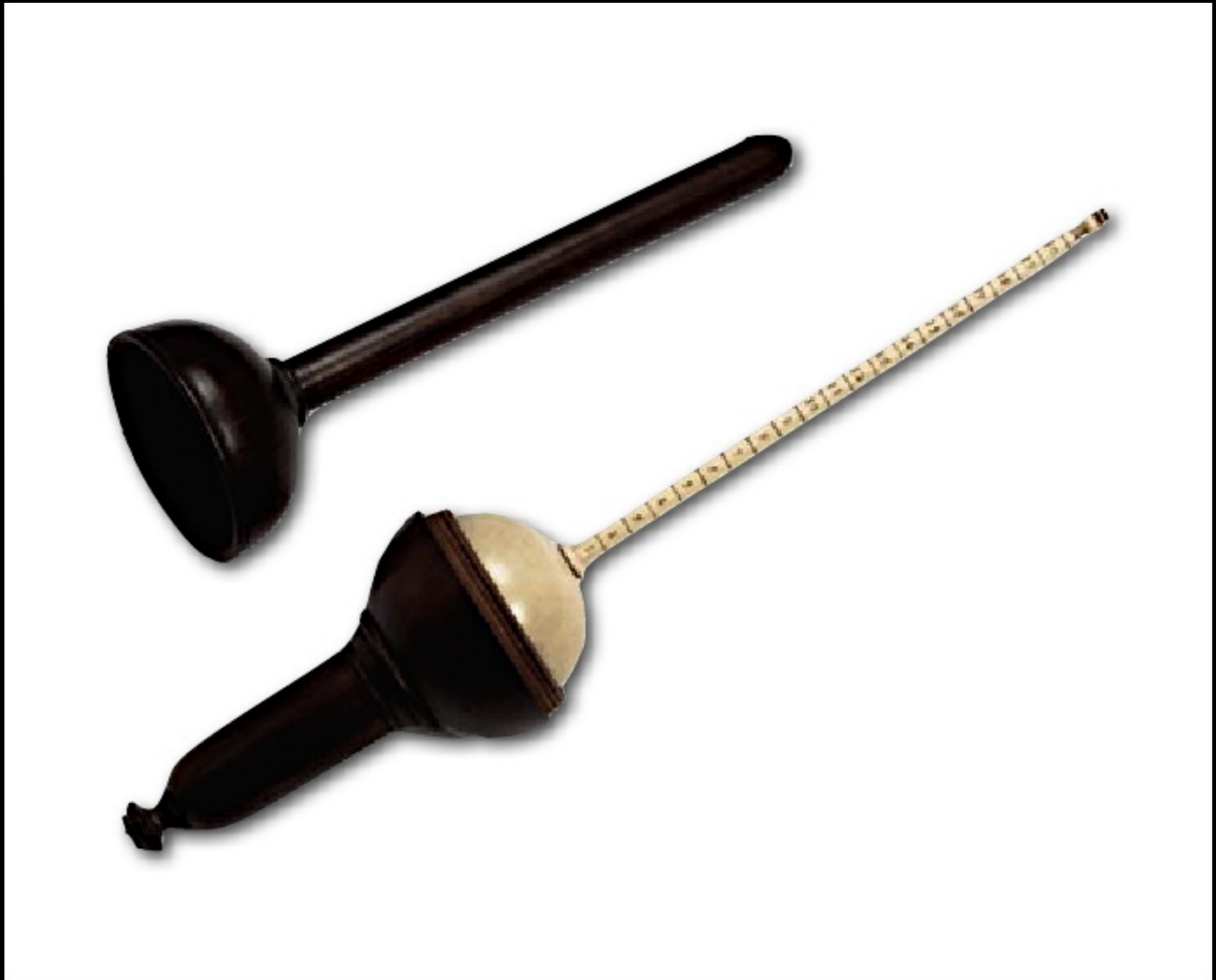
English Ivory, Lead, & Lignum Vitae Hydrometer to Measure the Density & Alcohol Content of Liquids for Taxation Purposes Late 18th Century (National Museums of Scotland)
