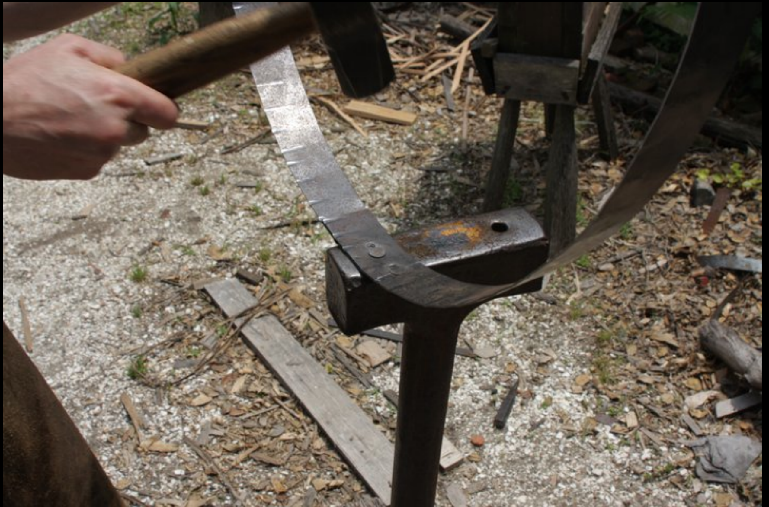
Driving a Rivet Through a Recreated Hoop Iron (The Colonial Williamsburg Cooperage - Colonial Williamsburg)
