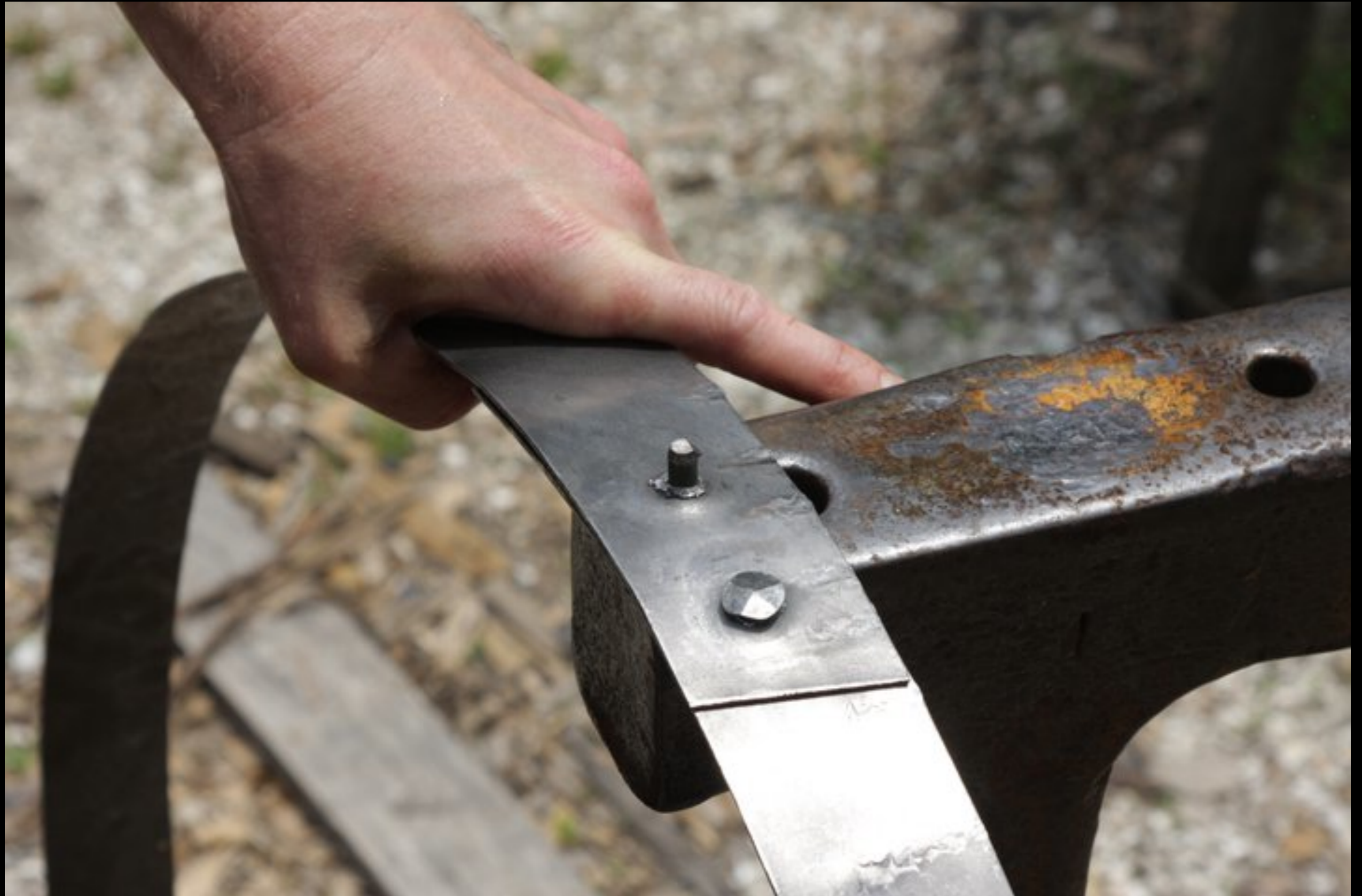
The Protruding Rivet Shank (The Colonial Williamsburg Cooperage - Colonial Williamsburg)
