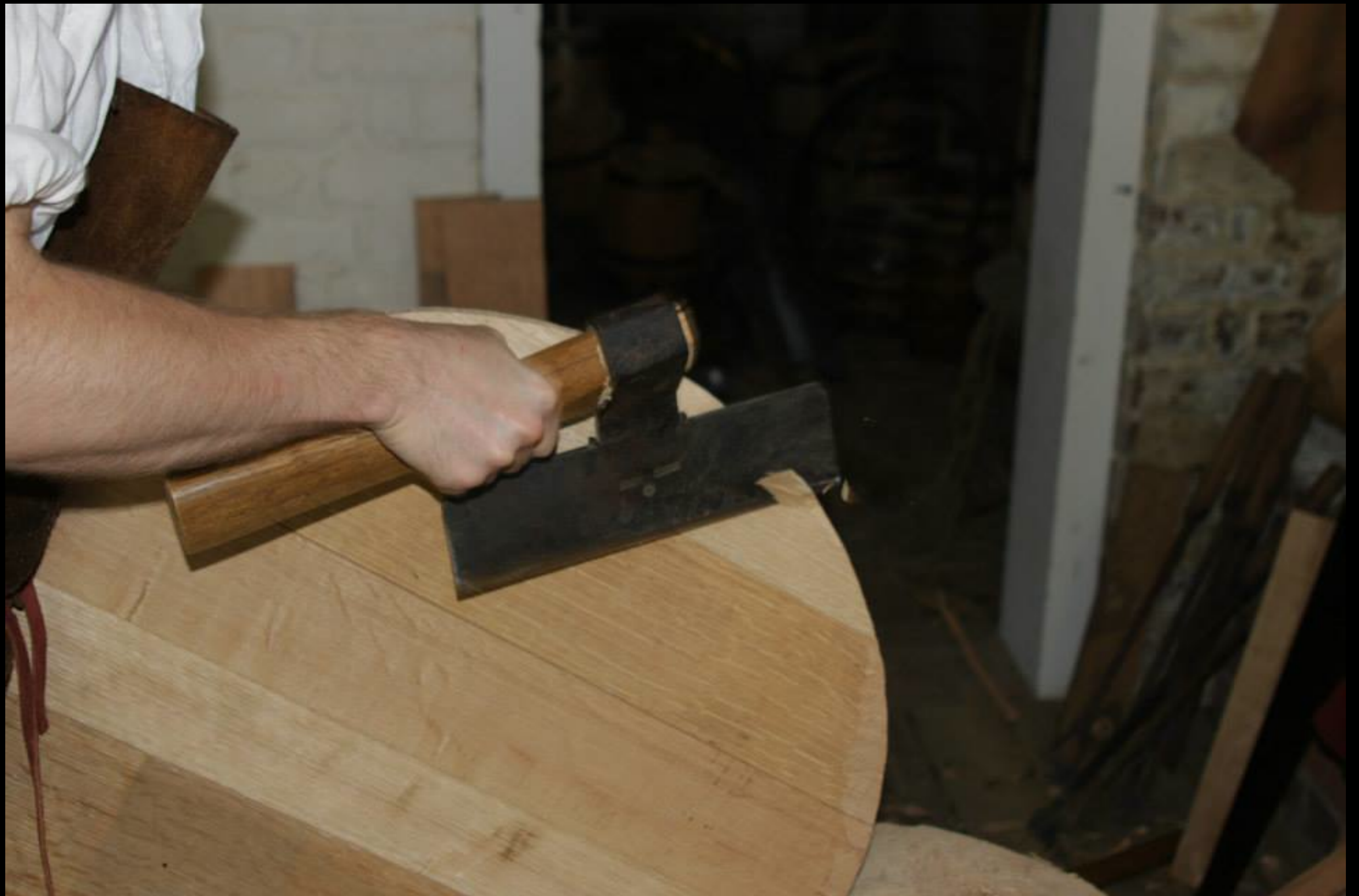
Using a Cooper's Axe to Cut a Bevel (The Colonial Williamsburg Cooperage - Colonial Williamsburg)
