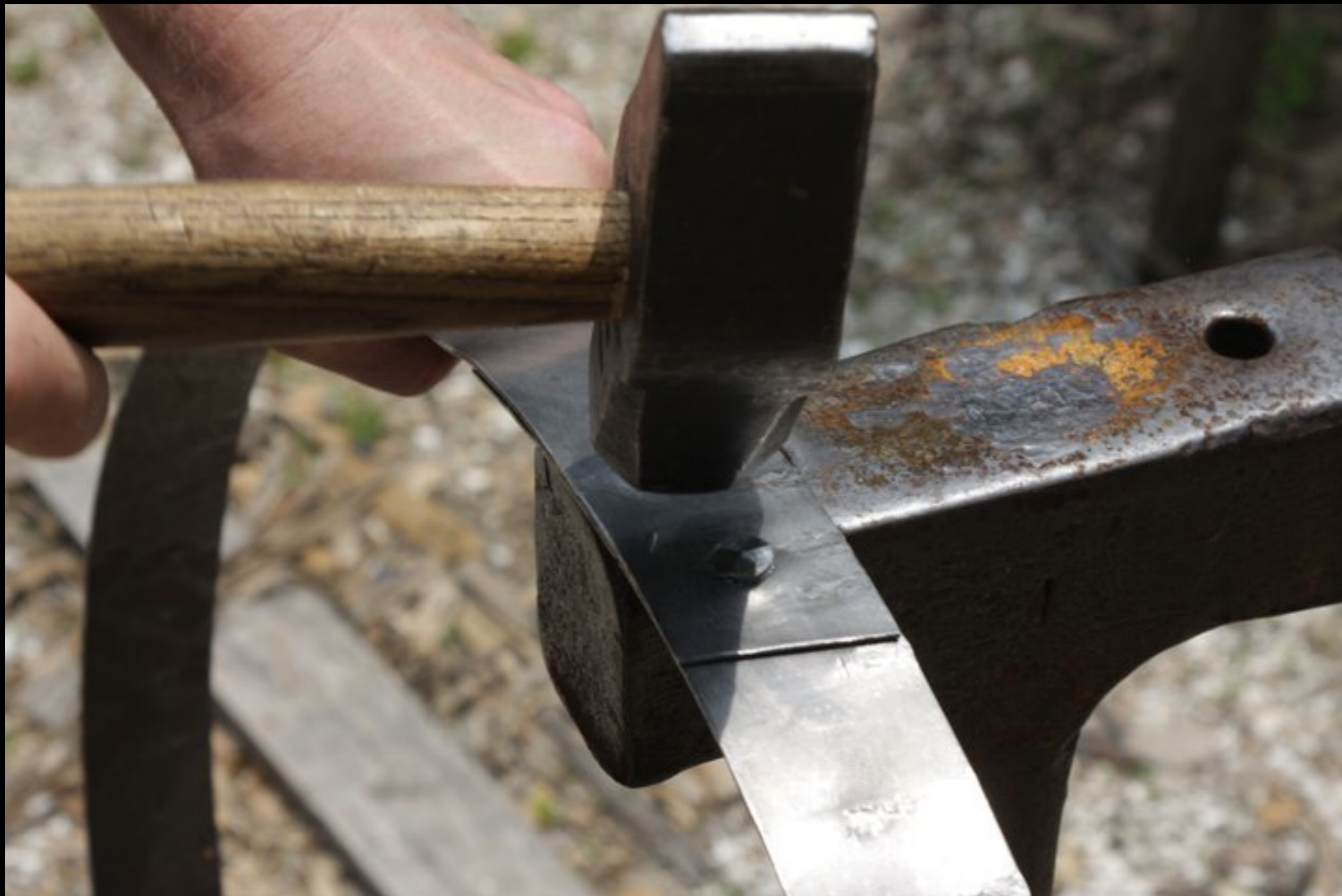
The Rivet Shank is Flattened into a Rosehead (The Colonial Williamsburg Cooperage - Colonial Williamsburg)
