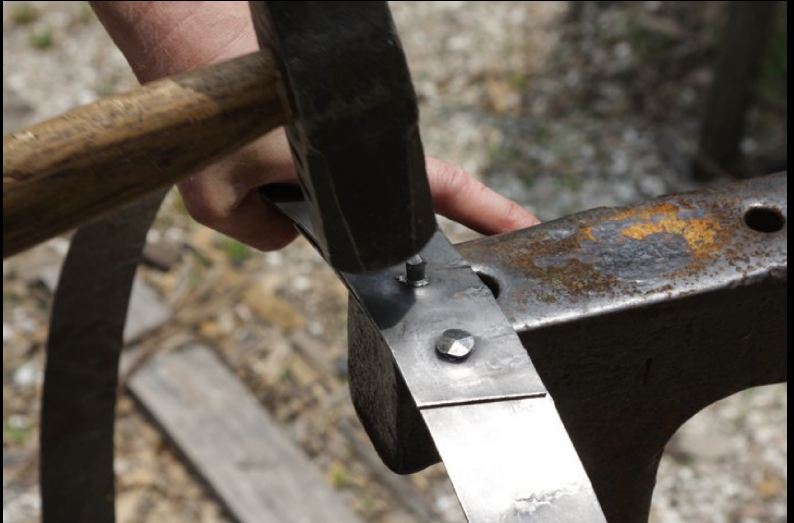
Hammering the Rivet Shank (The Colonial Williamsburg Cooperage - Colonial Williamsburg)
