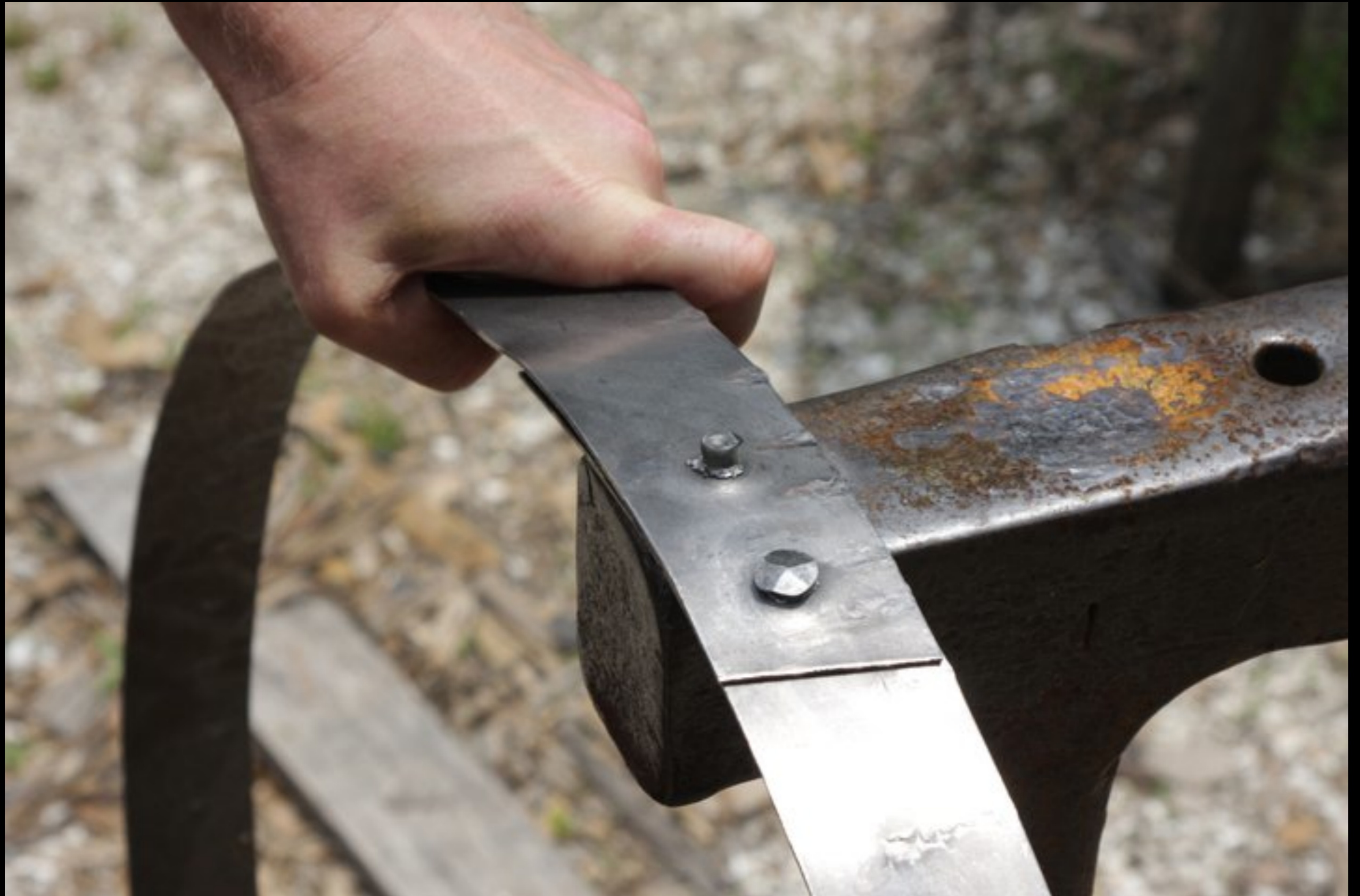
The Rivet Shank is Compressed (The Colonial Williamsburg Cooperage - Colonial Williamsburg)
