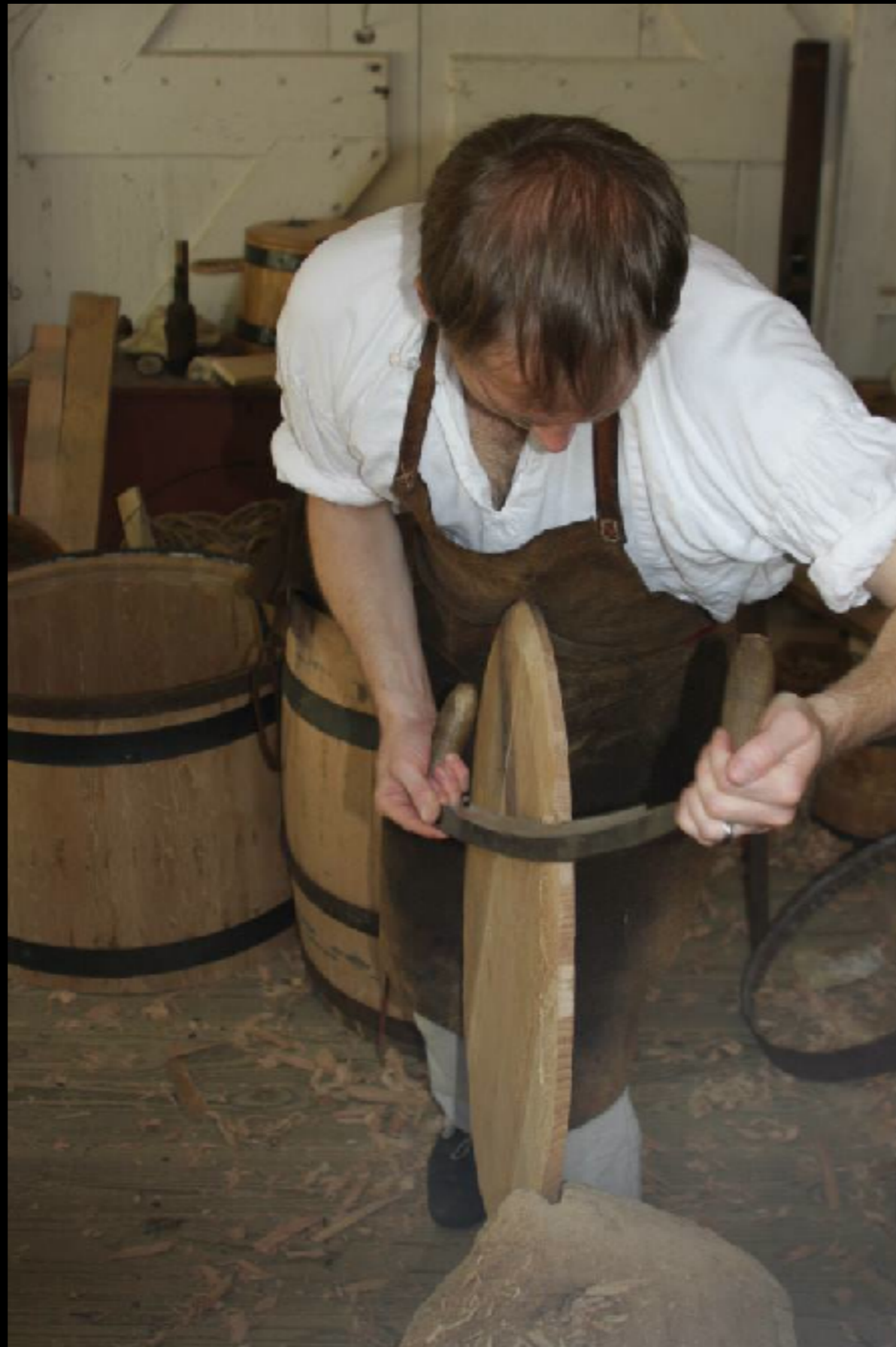
Finishing the Bevel with a Drawknife (The Colonial Williamsburg Cooperage - Colonial Williamsburg)
