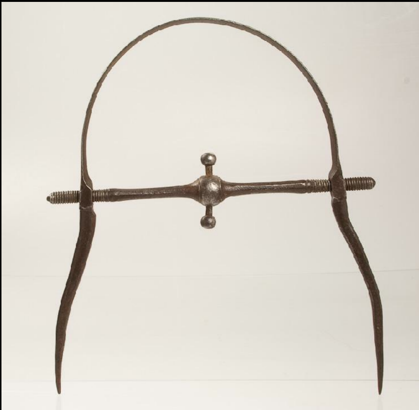
Coopers Dividers that Extend from 10" - 15" 17th - 18th Century (Jim Bode Historic Tools)
