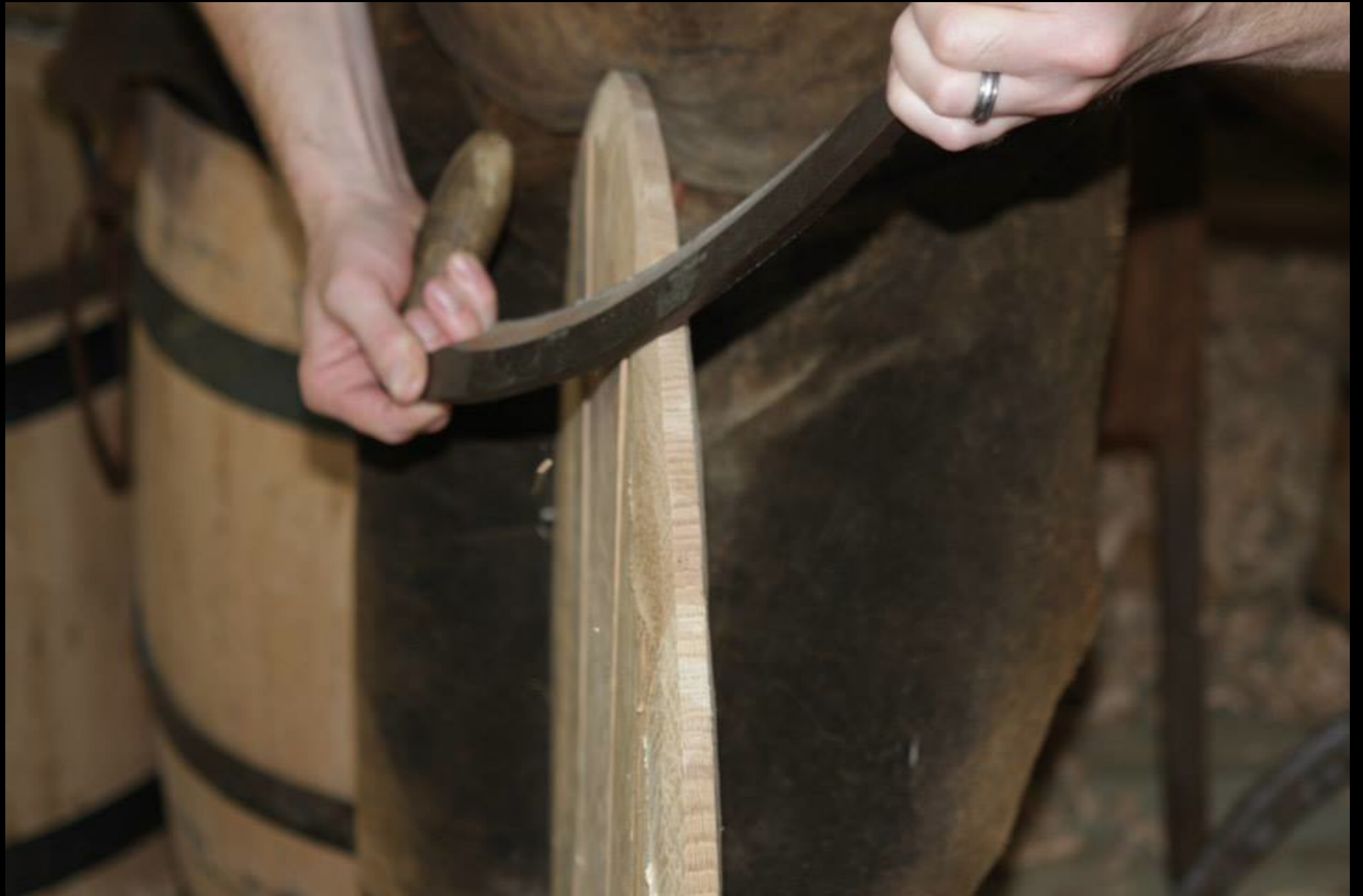
Finishing the Bevel with a Drawknife (The Colonial Williamsburg Cooperage - Colonial Williamsburg)
