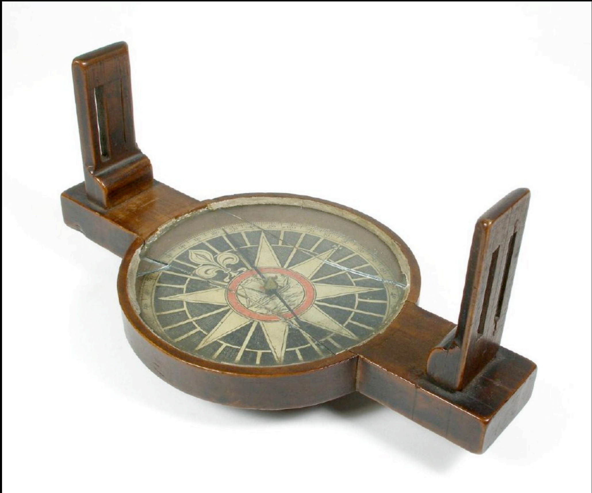
Surveyor's Compass by Joseph Halsey of Boston, Massachusetts c. 1750 - 1760 (New Hampshire Historical Society)
