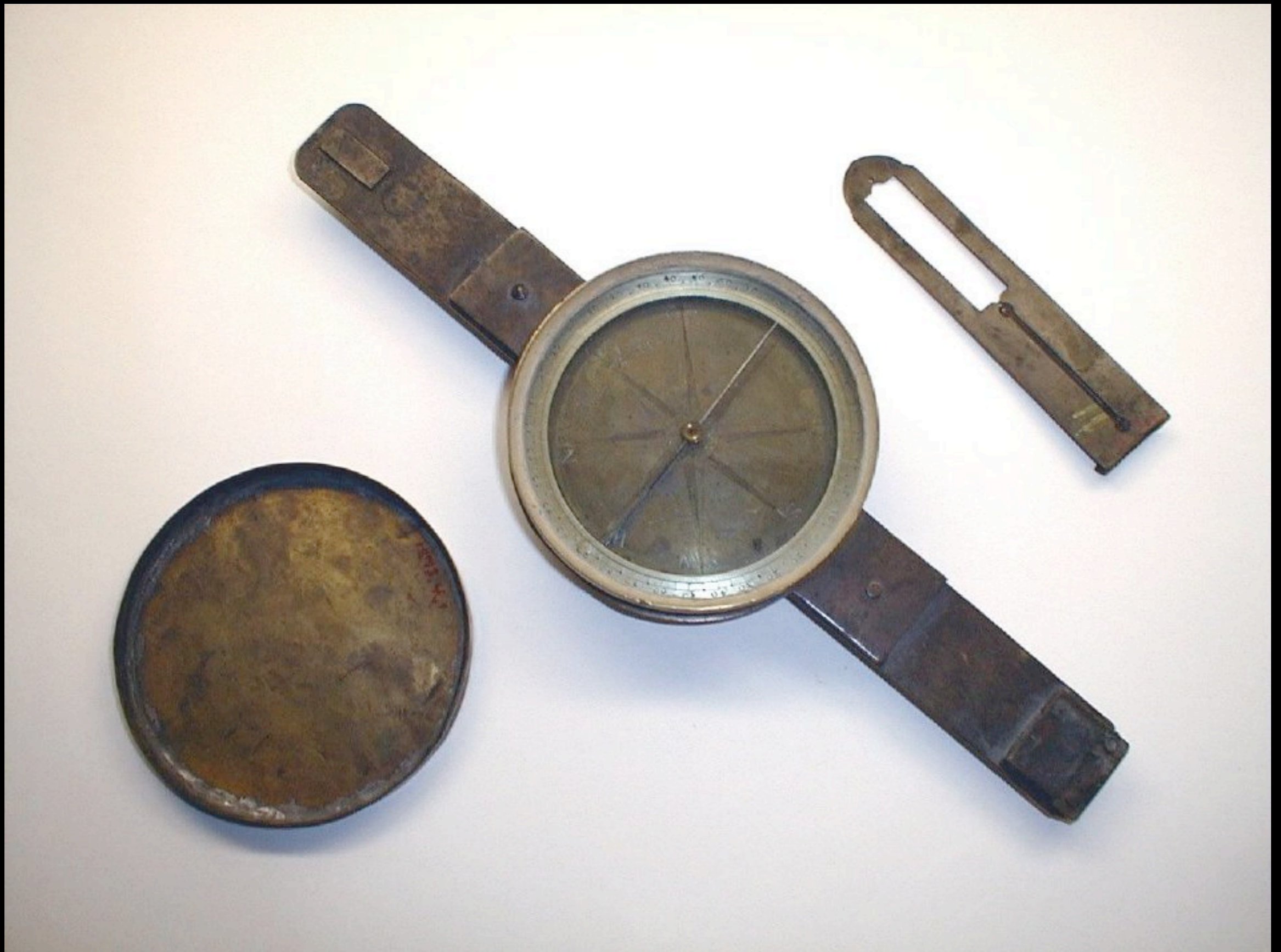
Surveyor's Compass by Stephen Greenleaf of Boston, Massachusetts c. 1750 (New Hampshire Historical Society)
