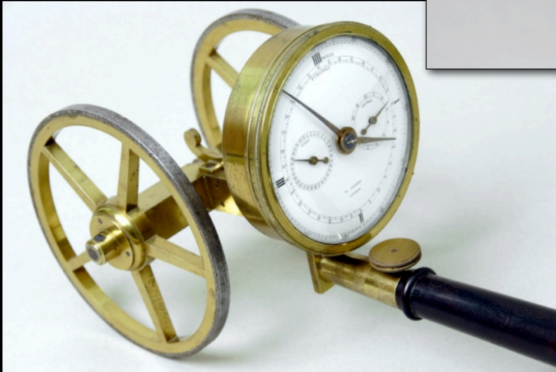
Waywiser or Perambulator by George Adams, Jr. (1750 - 1795) with Lock Patented by Joseph Bramah in 1784 (Scientific Instrument Society)
