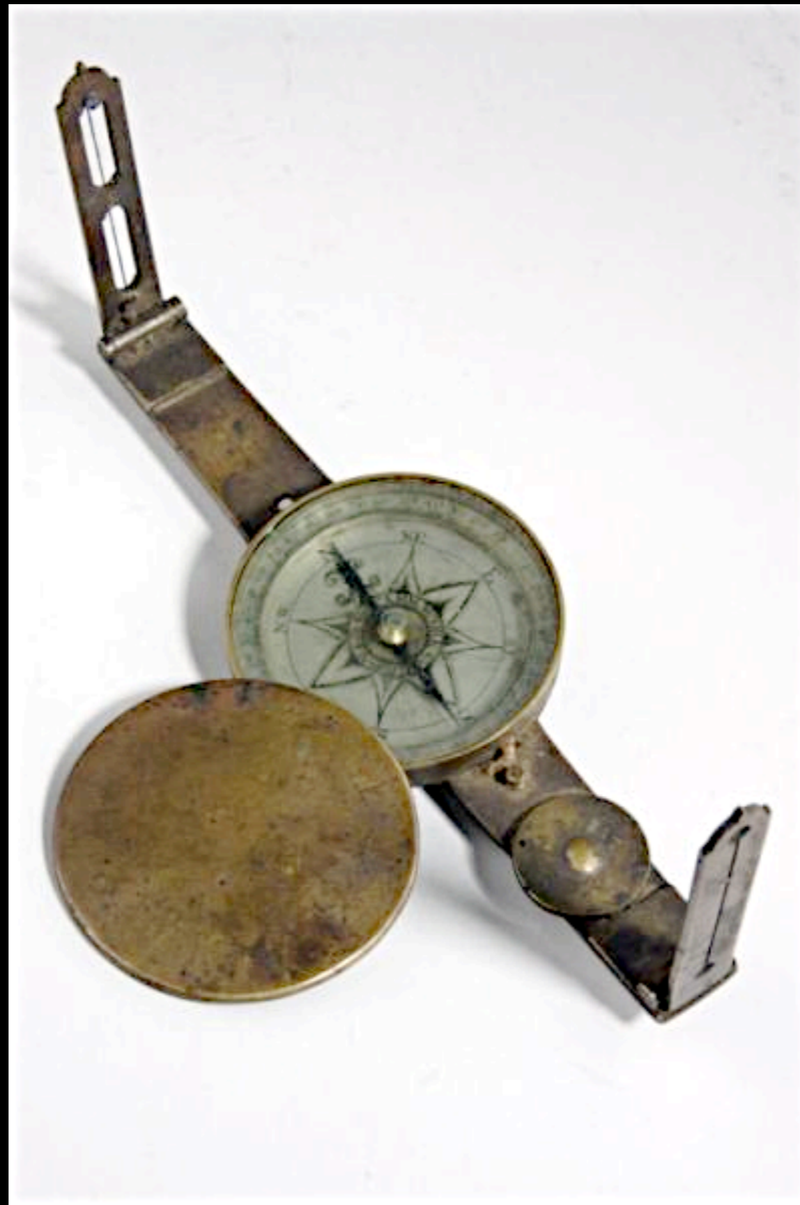
Surveyor's Compass by Camm Moore (1755 - 1845) of North Carolina (Leland Little Auction & Estate Sales)
