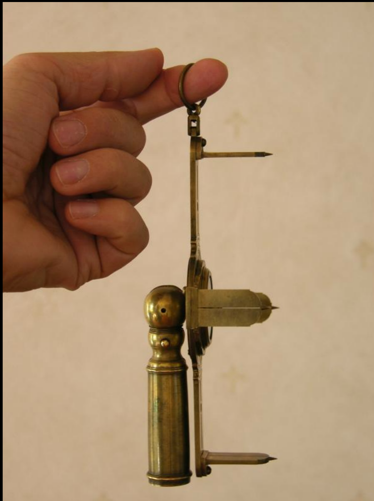
Surveyor's Cross or Graphometer Late 17th Century - 18th Century (Nicolàs de Hilster)
