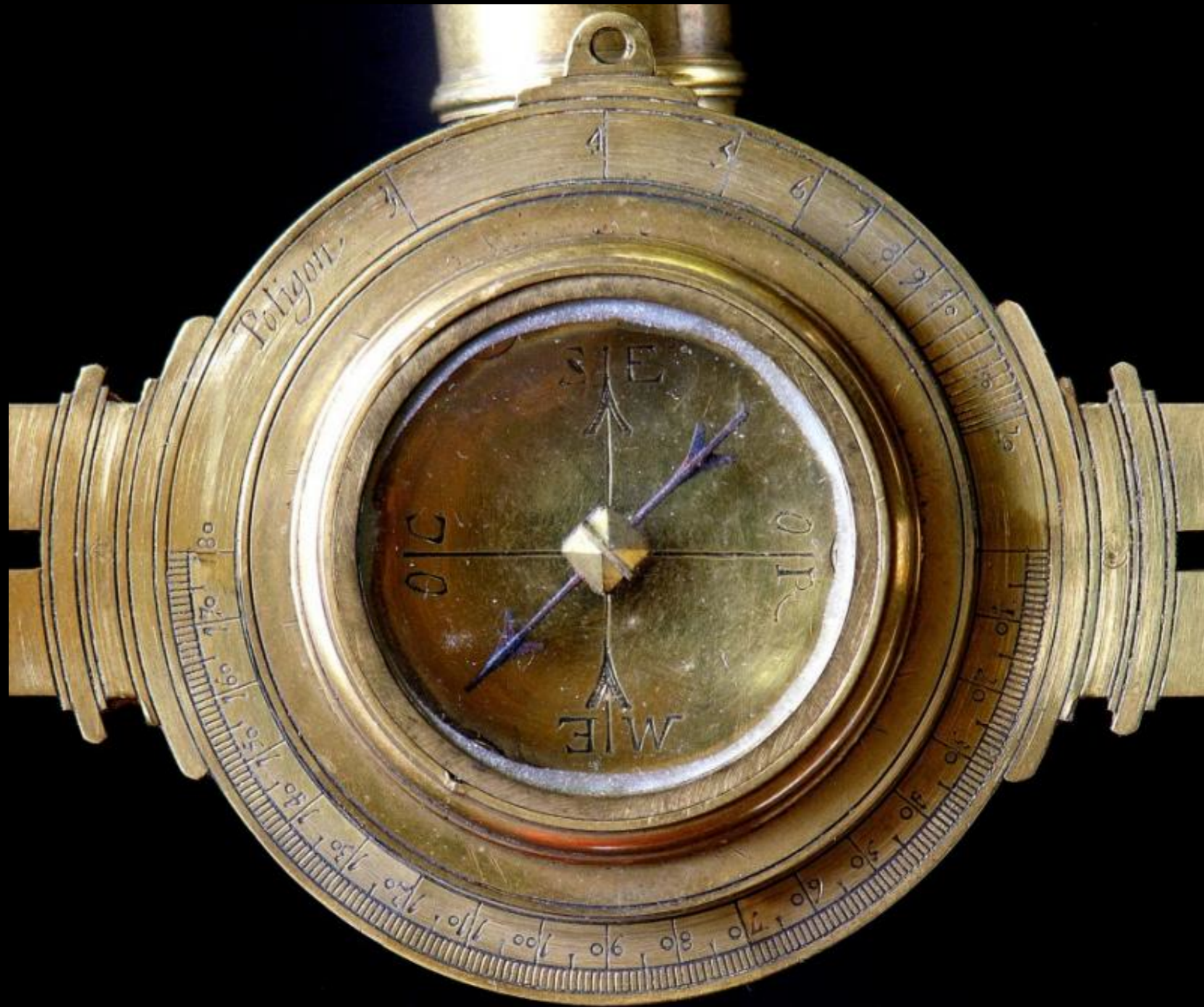
Surveyor's Cross or Graphometer Late 17th Century - 18th Century (Nicolàs de Hilster)
