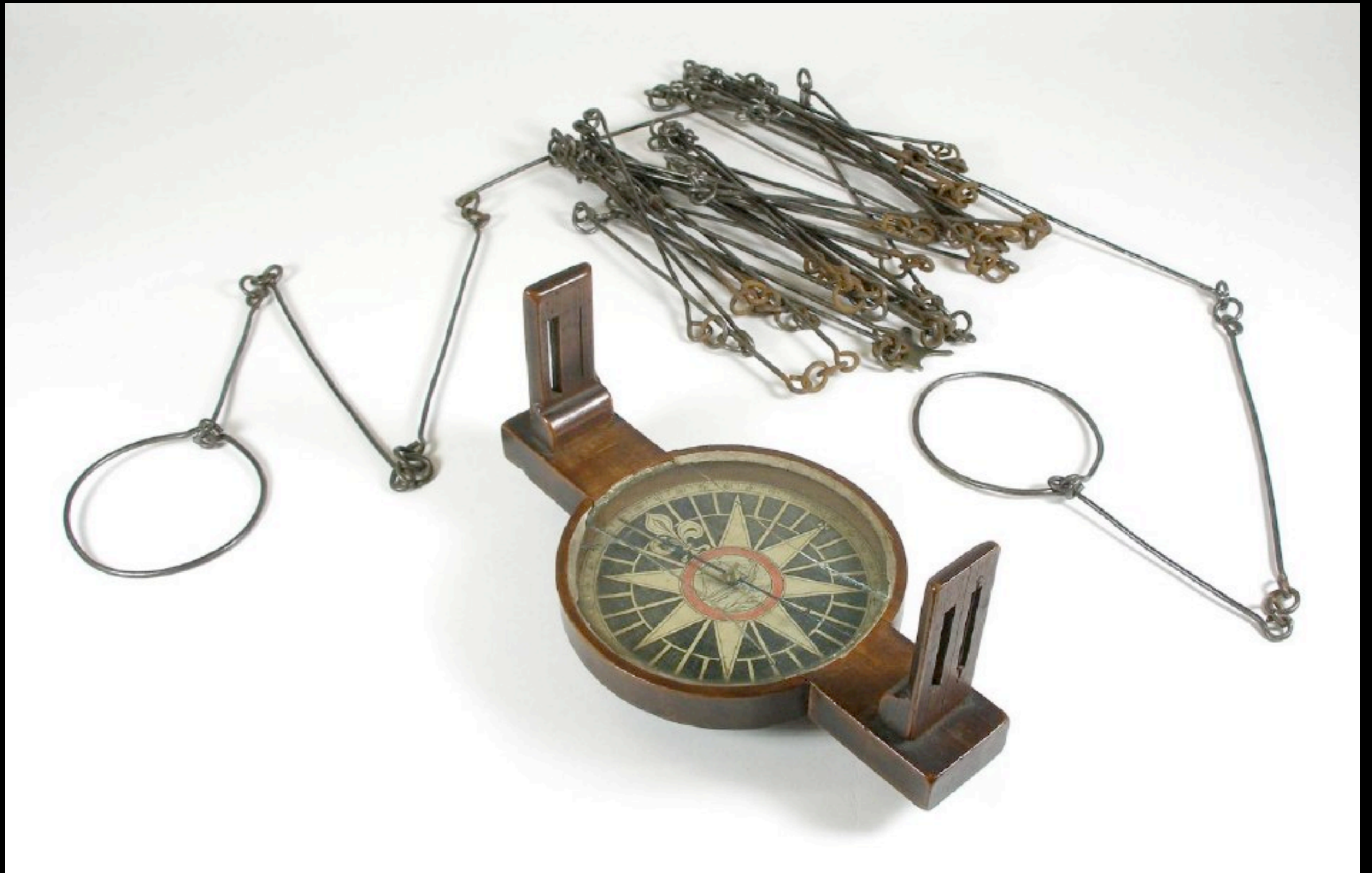
Surveyor's Compass & Chain by Joseph Halsey of Boston, Massachusetts c. 1750 - 1760 (New Hampshire Historical Society)
