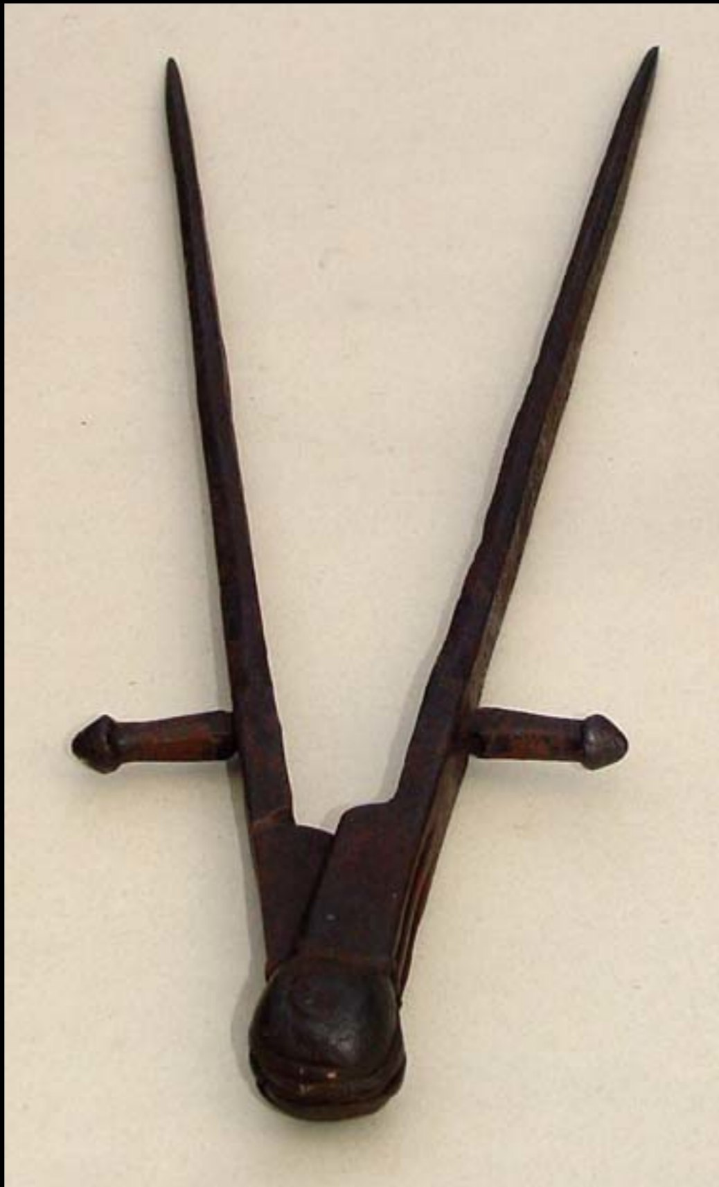
European Wrought Iron Dividers Late 17th - 18th Century (Tesseract - Early Scientific Instruments)
