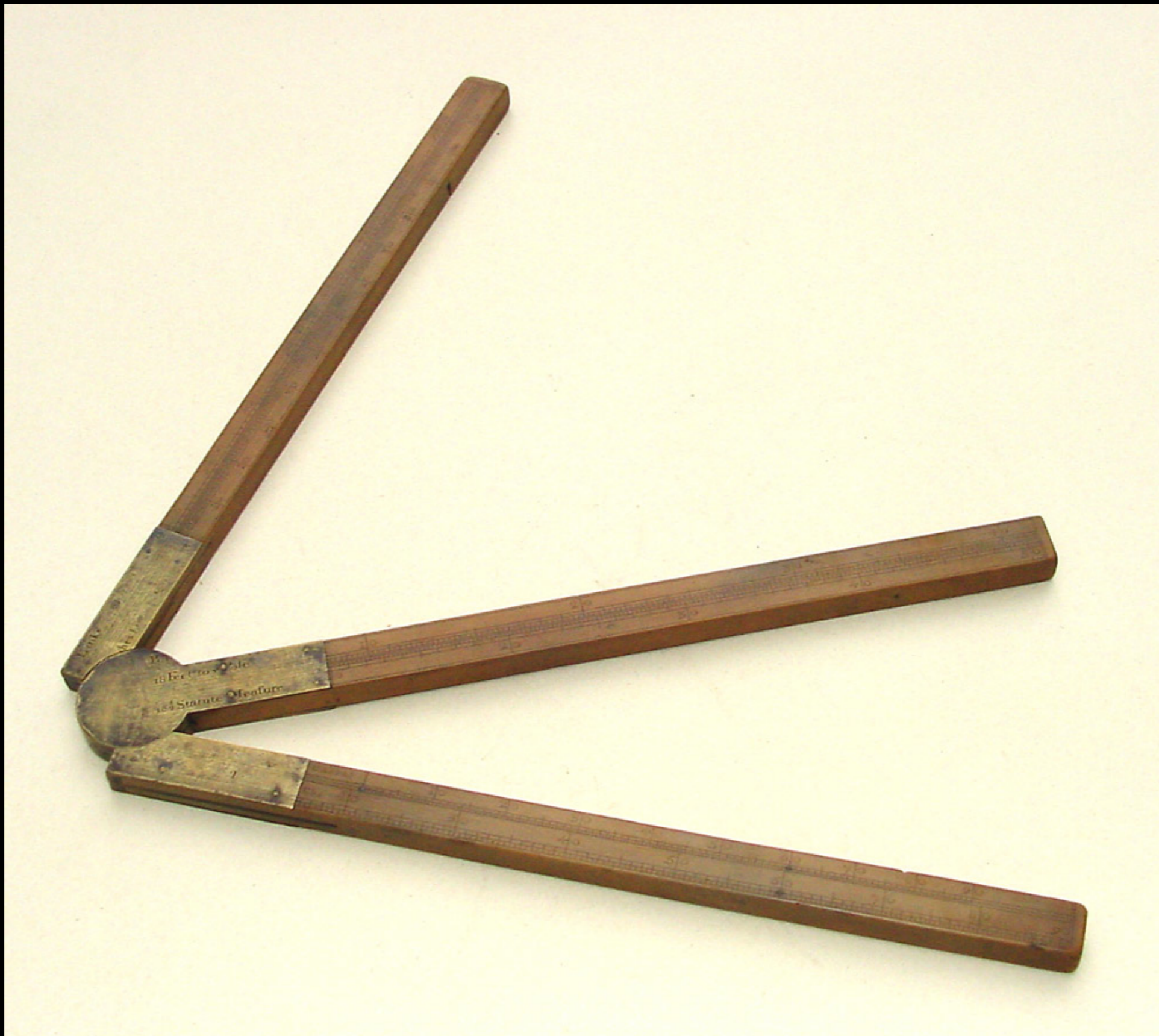
English Surveyor's Boxwood Three Arm Conversion Rule First Half 18th Century (Tesseract - Early Scientific Instruments)
