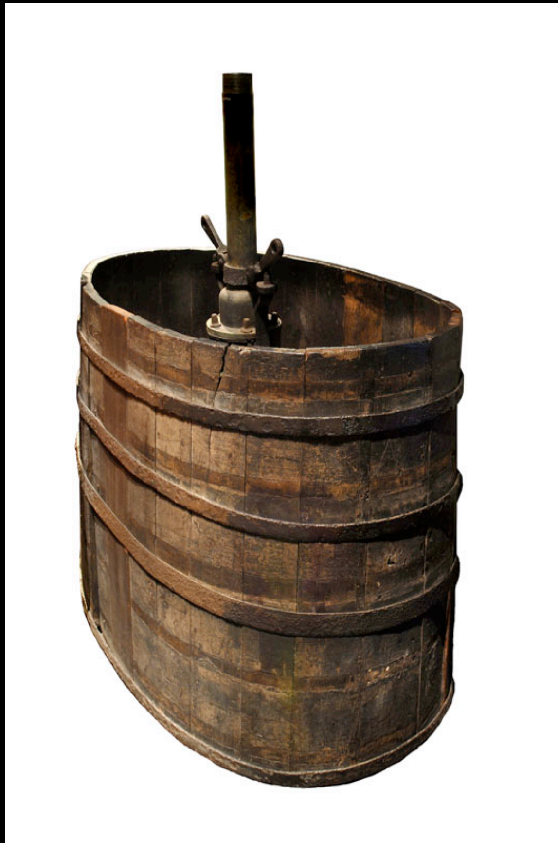
Fire Engine made by John Keeling of Blackfriars in 1678 (Wheels and Arms of the Pump are Missing) (Museum of London)
