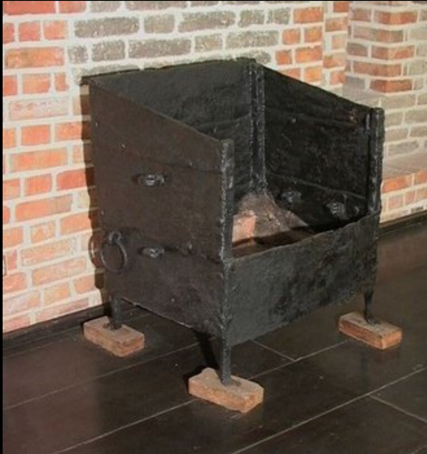
English Cast Iron Ship Stove Recovered from the Wreck of the General Carleton c. 1785 (Polish National Maritime Museum)
