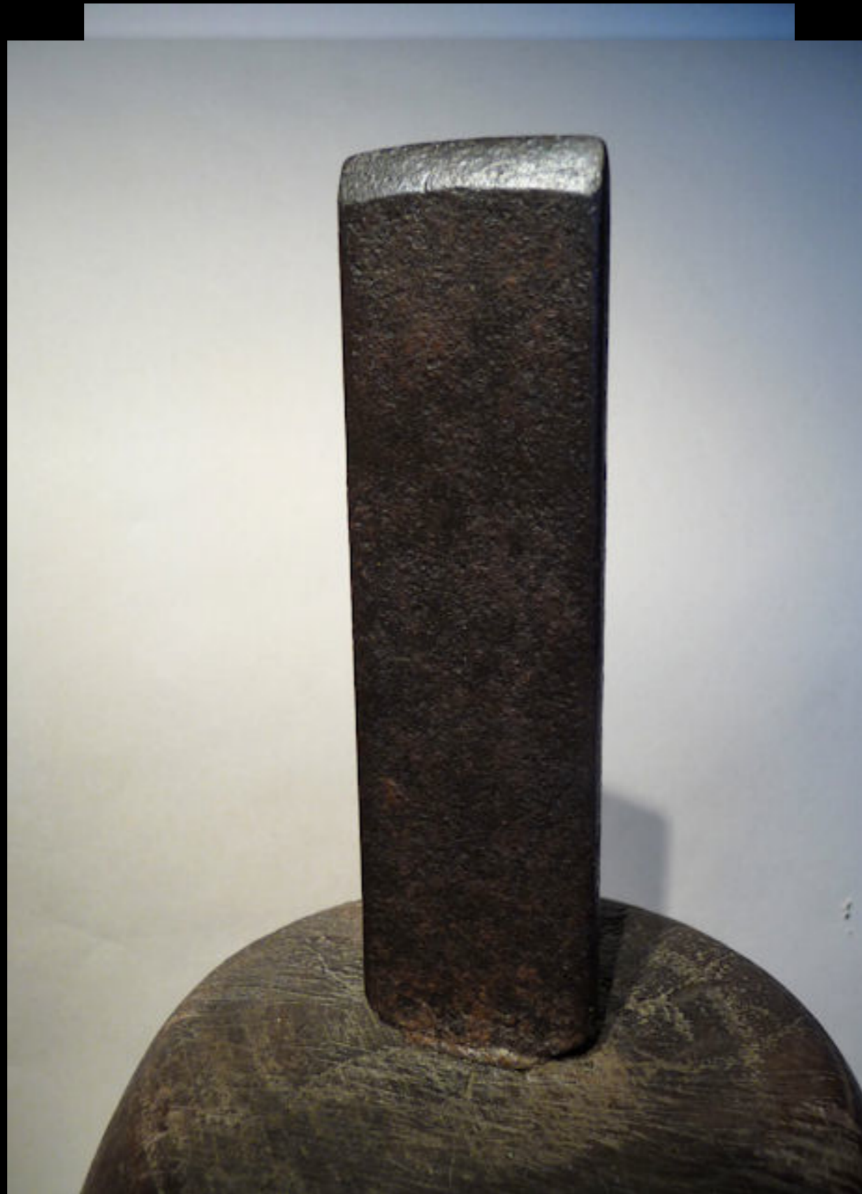
New England Oyster Shucker Wrought Iron Blade into a Wooden Base (Sharon Platt)
