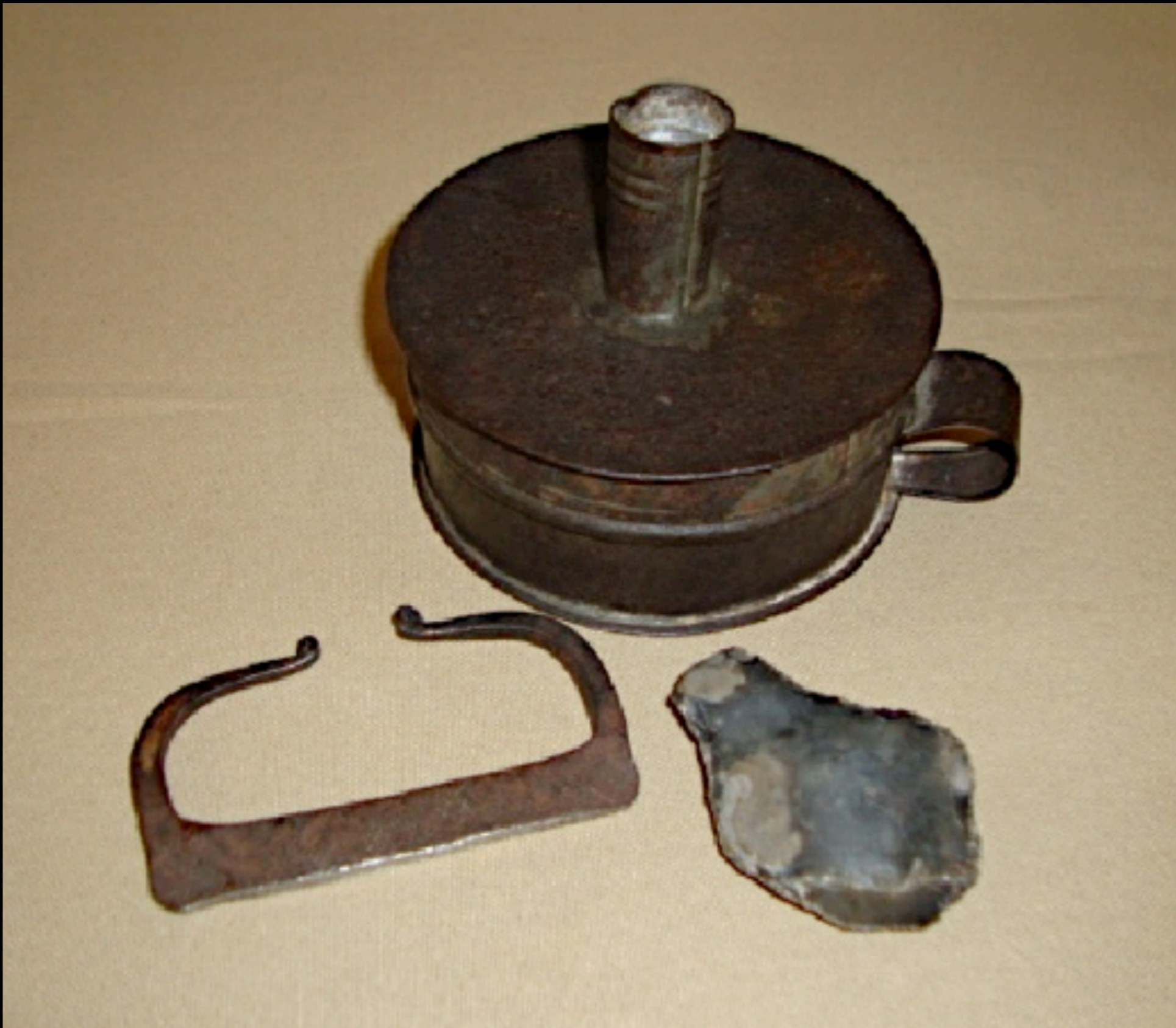
Tinned Iron Tinder Box & Striker Late 18th Century - Early 19th Century (Antiques of Early America)
