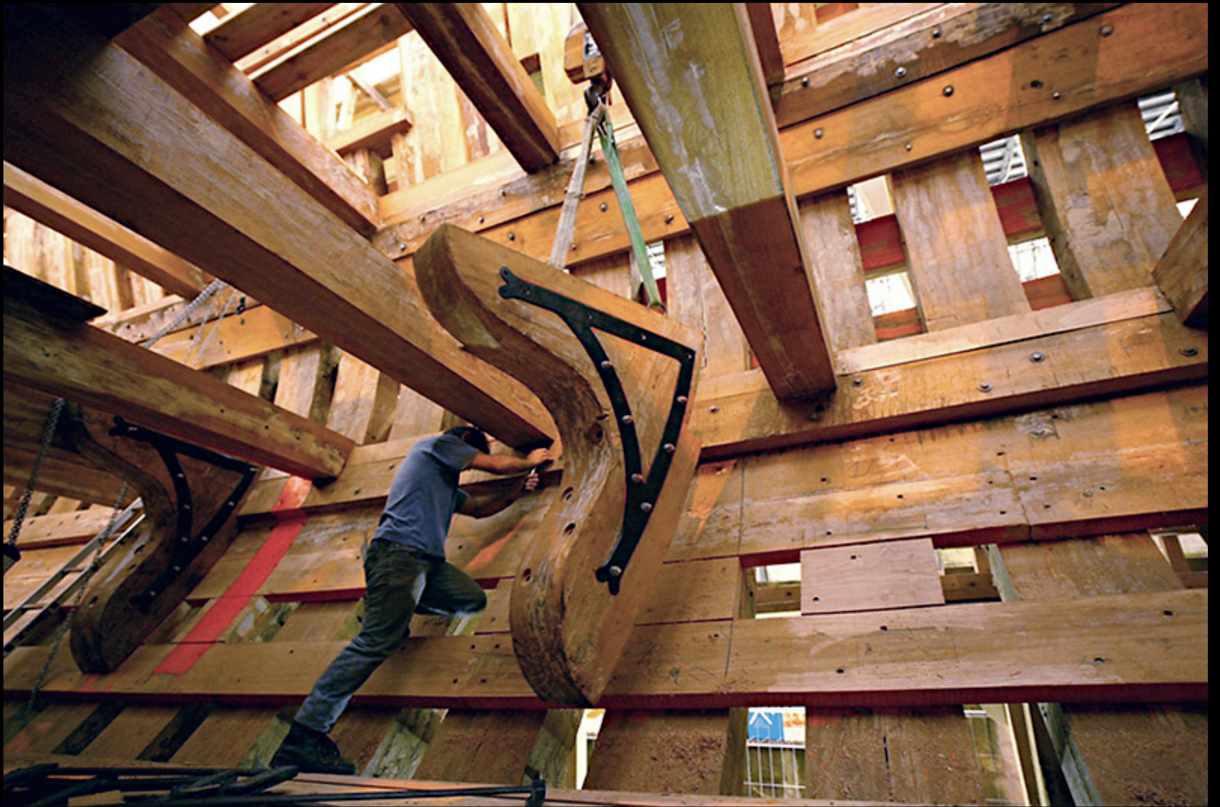
Reconstructing L'Hermione - Rochefort, France
