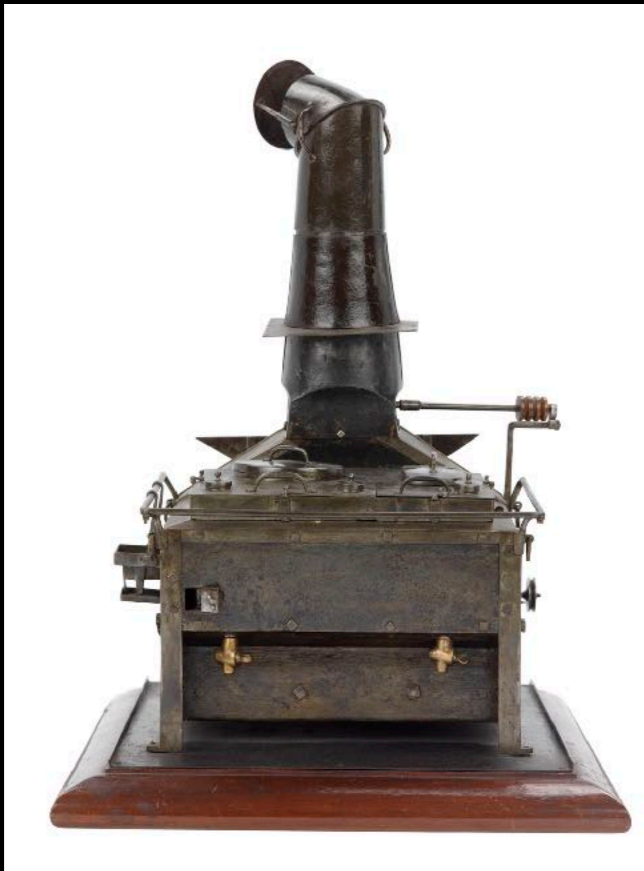
English Model of a Brodie "New Ship Stove, Kitchen, or Hearth, with a Smoak Jack and Iron Boilers..." by George Cawthorn Patented by Alexander Brodie of Carey Street, Middlesex. Stoves in 1780. Used on Royal Navy Ships in 1781 c. 1780 (National Maritime Museum, Greenwich)
