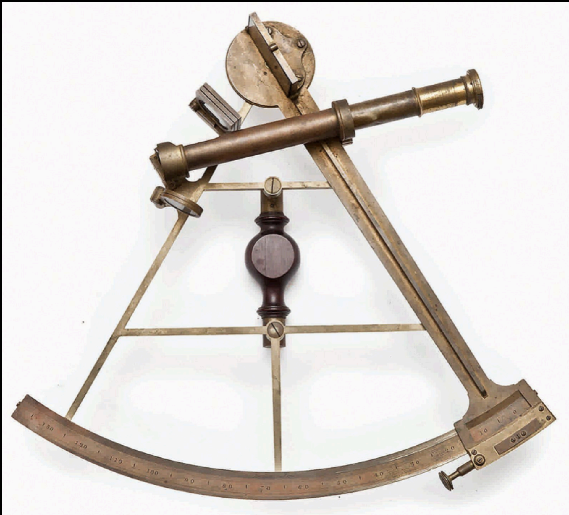
English 12 Inch Brass Vernier Octant by Jesse Ramsden c. 1785 (Charles Miller Ltd.)
