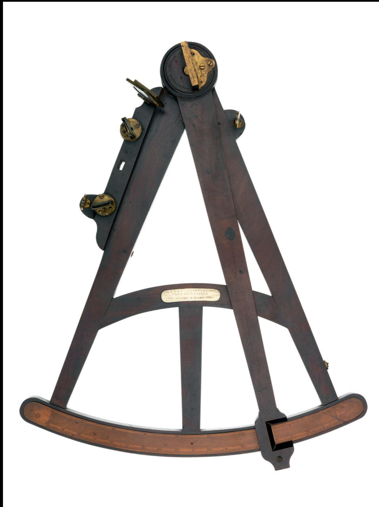
English Mahogany & Boxwood Octant by Thomas Lake of London c. 1770 (National Maritime Museum, Greenwich)
