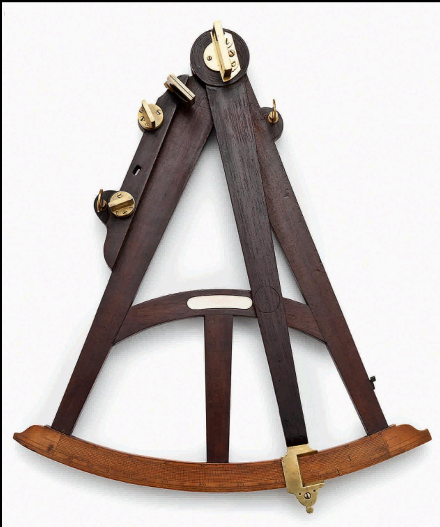
English 17 \frac{1}{2} Inch Radius Boxwood Fiducial Octant from London c. 1780 (Charles Miller Ltd.)
