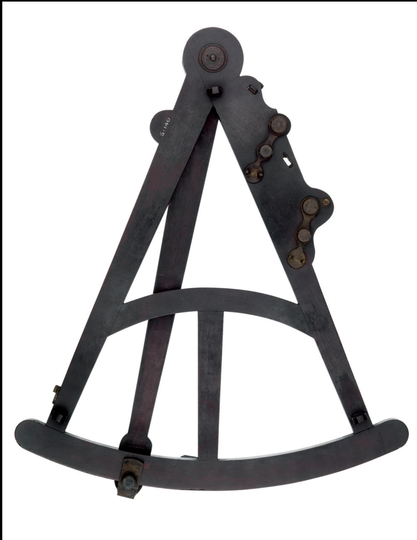
English Mahogany & Boxwood Octant by Benjamin Cole of London c. 1750 (National Maritime Museum, Greenwich)
