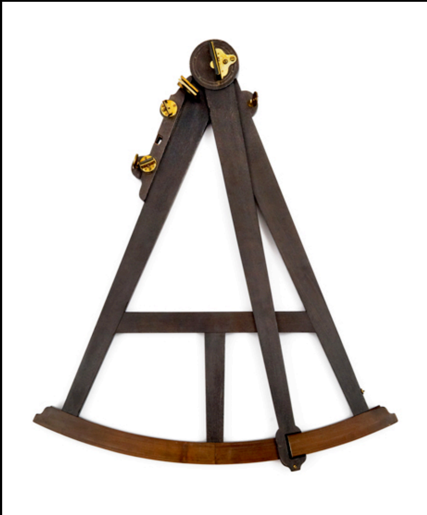
English 23\frac{1}{2} Inch Radius Ebony & Boxwood Octant by Edward Nairne of London c. 1760 (Charles Miller Ltd.)
