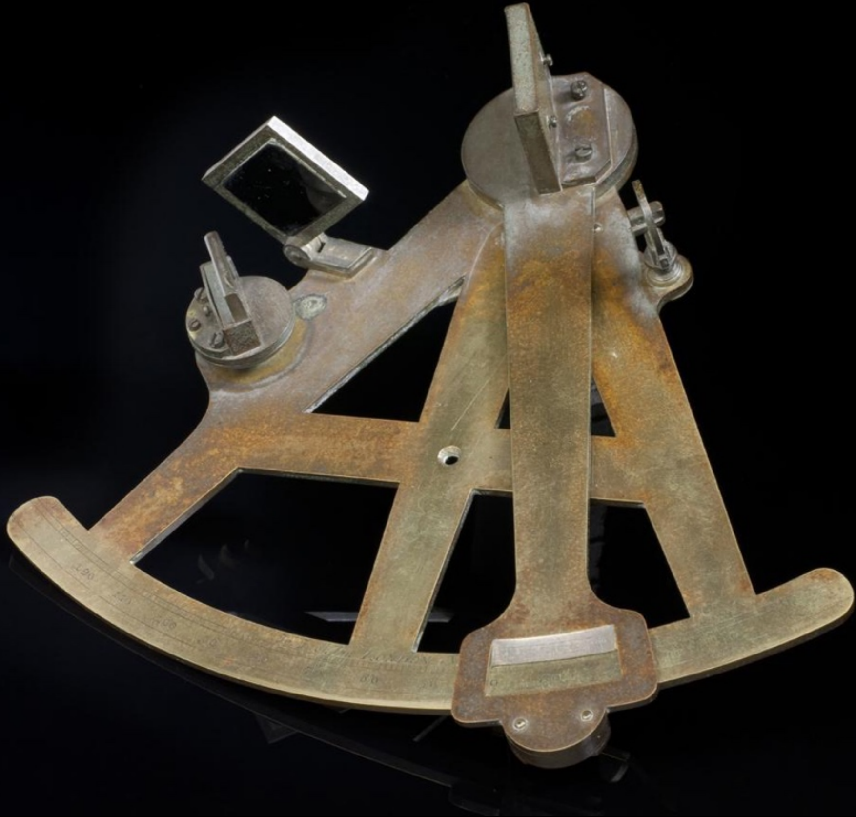
English 5 1/2 Inch Radius Brass Vernier Sextant by Joseph Jackson of London c. 1757 - 1762 (Museum of Science and Industry, Manchester)
