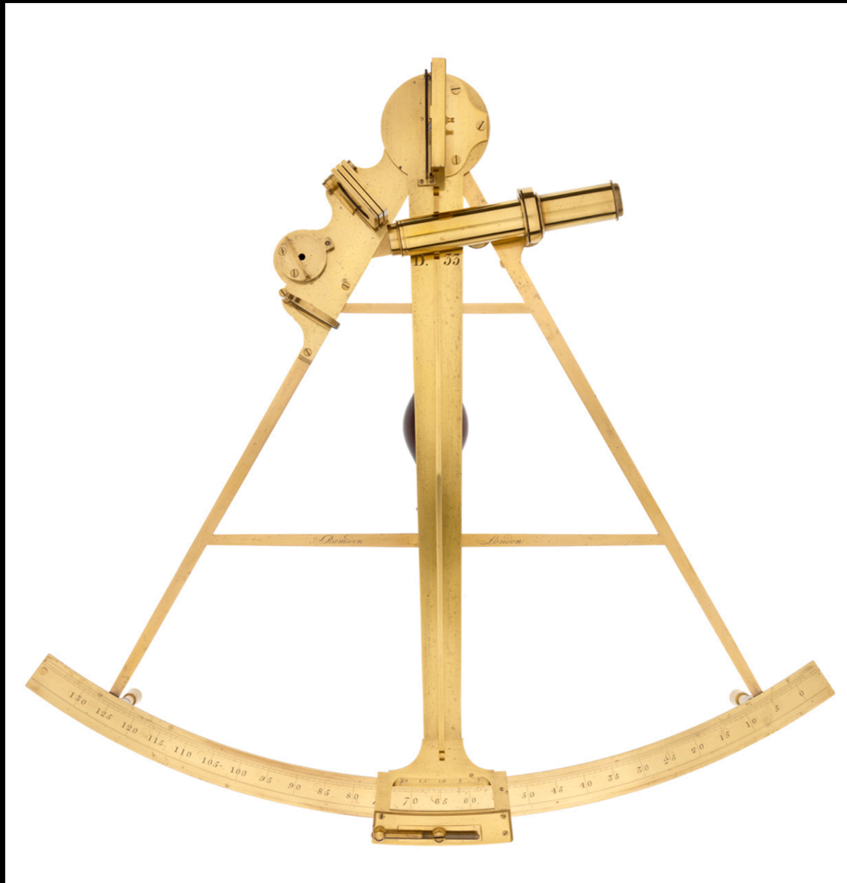
English Brass Sextant by Jesse Ramsden of London 1772 (National Maritime Museum, Greenwich)
