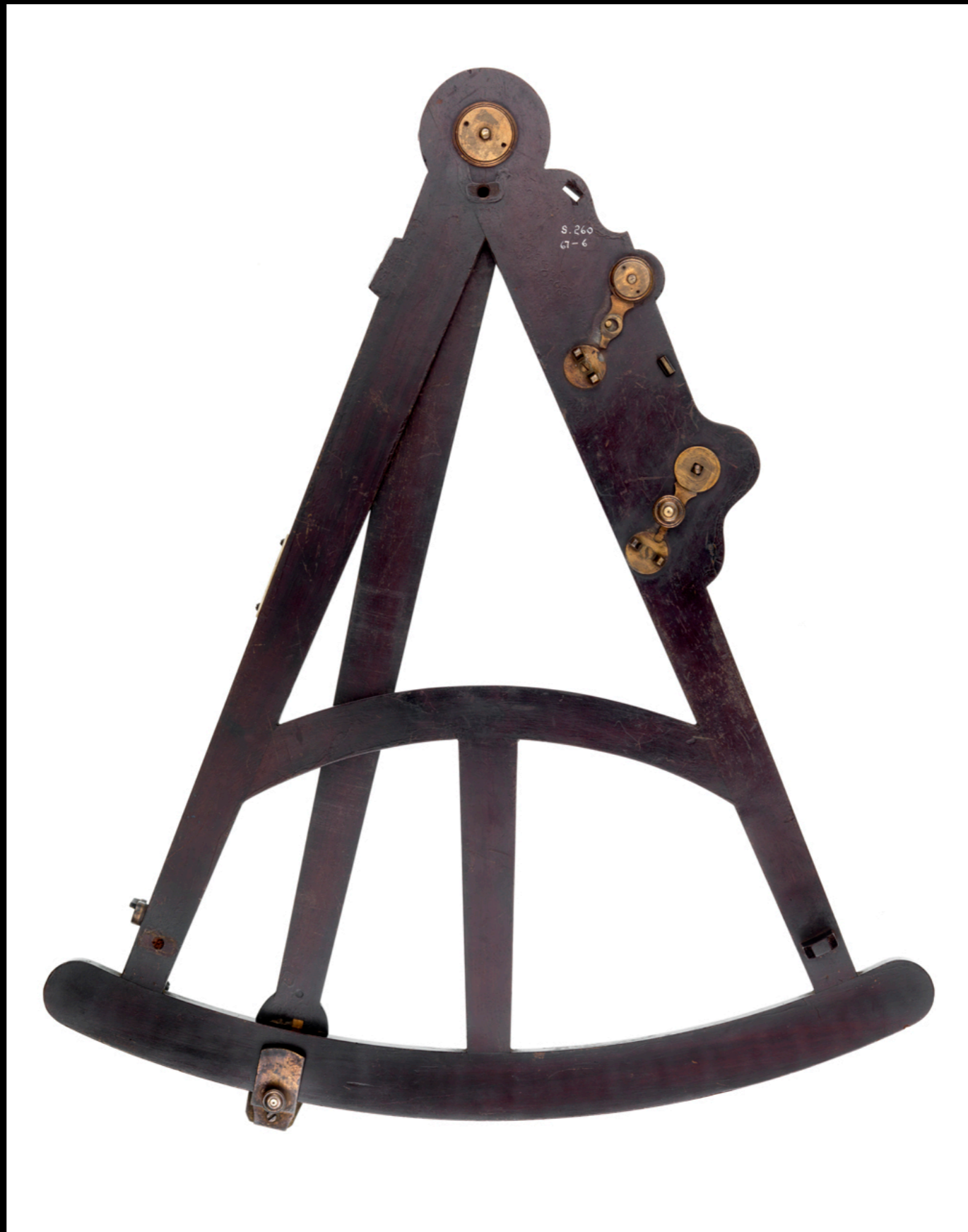
English Mahogany & Boxwood Octant by Benjamin Cole of London c. 1760 (National Maritime Museum, Greenwich)
