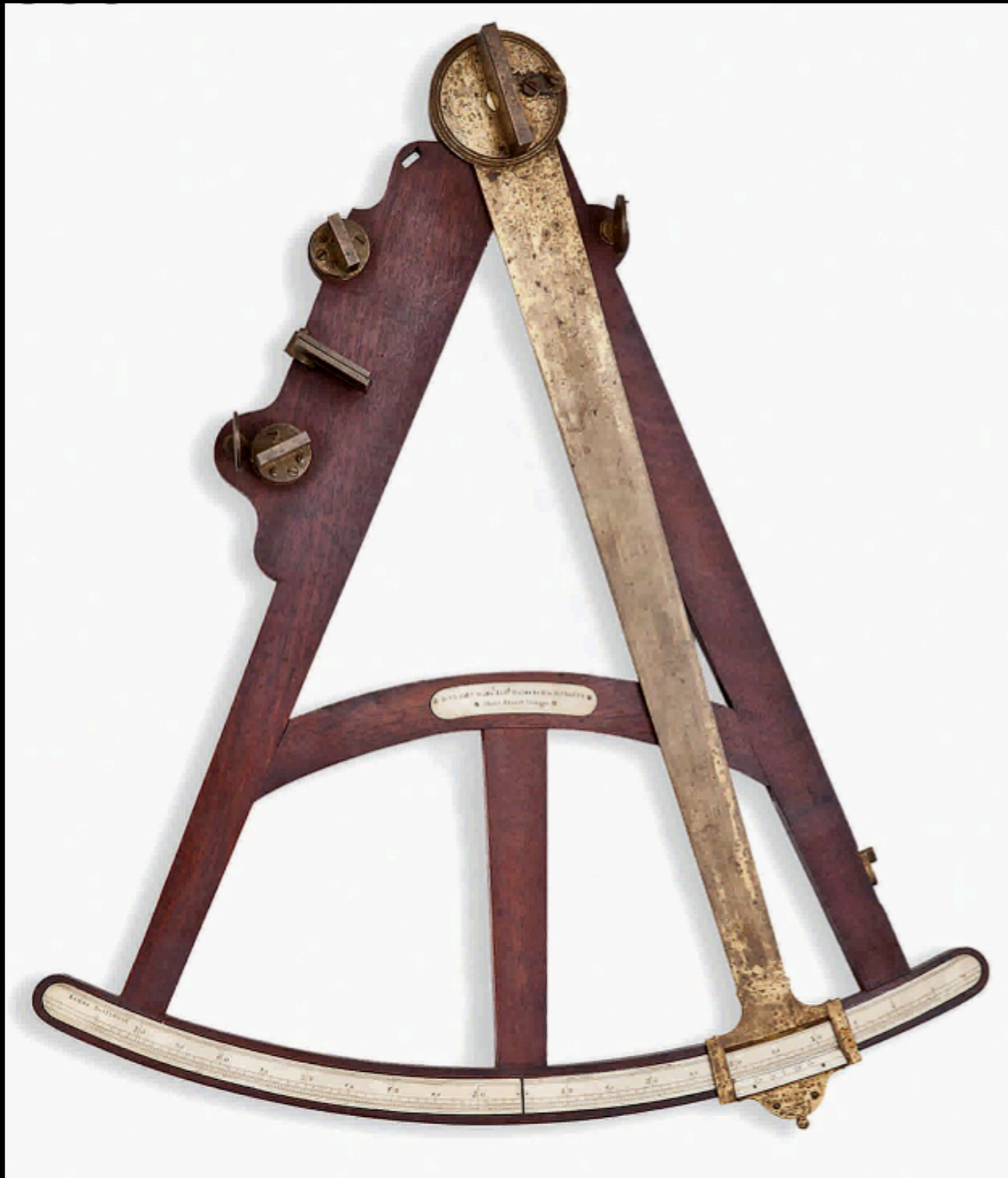
English 17 Inch Mahogany & Ivory Vernier Octant Inscribed to James Smallwood “G. ADAMS Mathl. Inst. Maker to His MAJESTY / Fleet Street London” c. 1770 (Charles Miller Ltd.)
