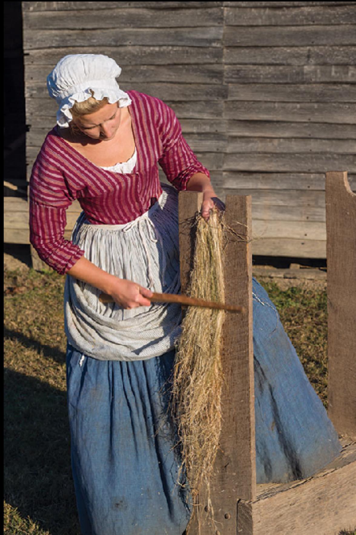
Flax Processing - Beating the Flax and Separating the Waste from the Long Fibers with a Scutching Board or Brake and Knife (Colonial Williamsburg Foundation - Dave Dooly Photograph - From "Flax & Hemp in Colonial America" by Ben Swenson)
