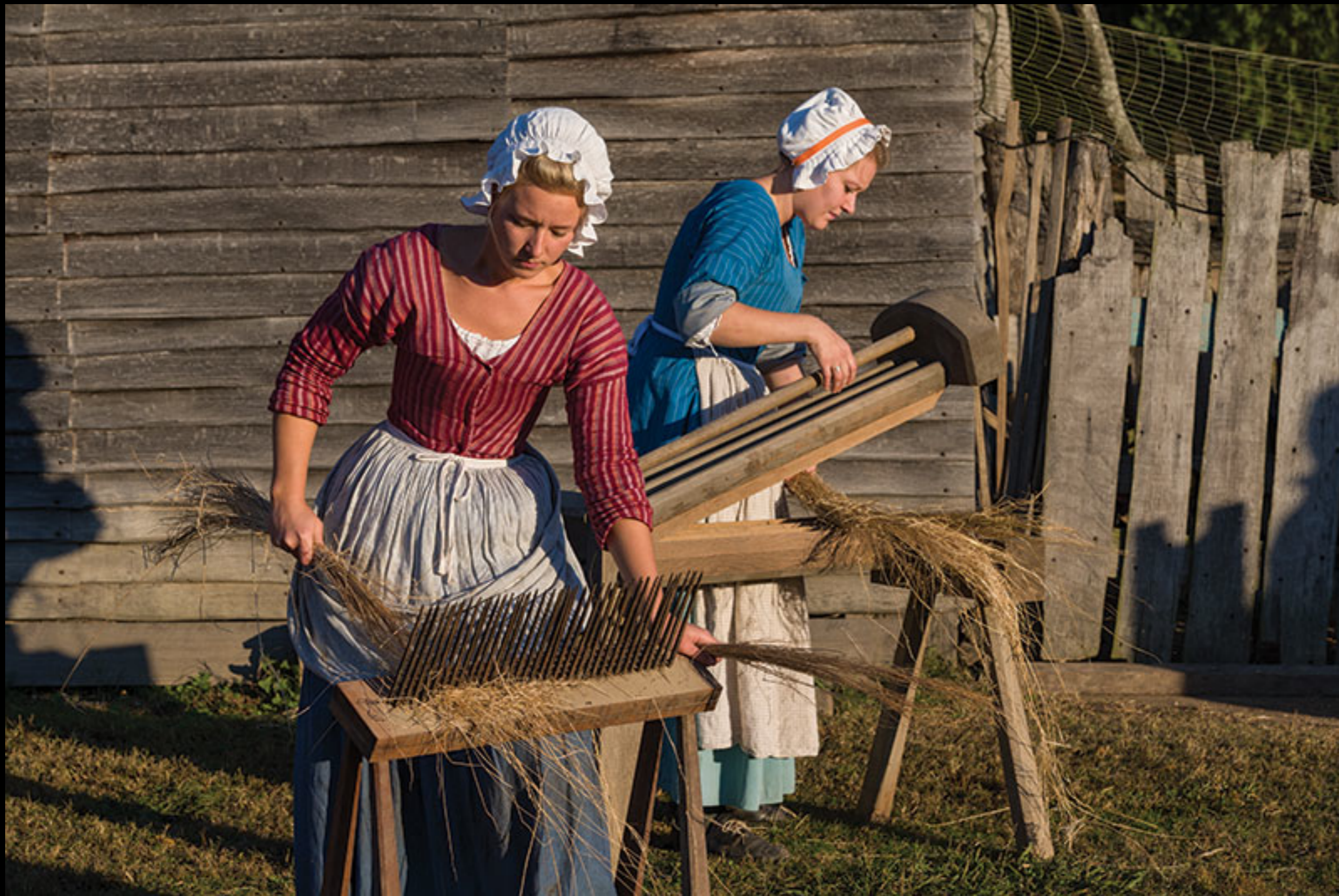
Flax Processing - Initial Removal of the Flax Seeds and Straw Bark with a Ripple after Crushing (Colonial Williamsburg Foundation - Dave Dooly Photograph - From "Flax & Hemp in Colonial America" by Ben Swenson)
