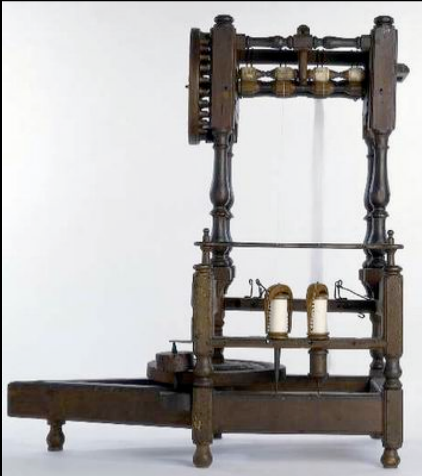
Sir Richard Arkwright's Prototype Spinning Machine England 1769 (SCM)
