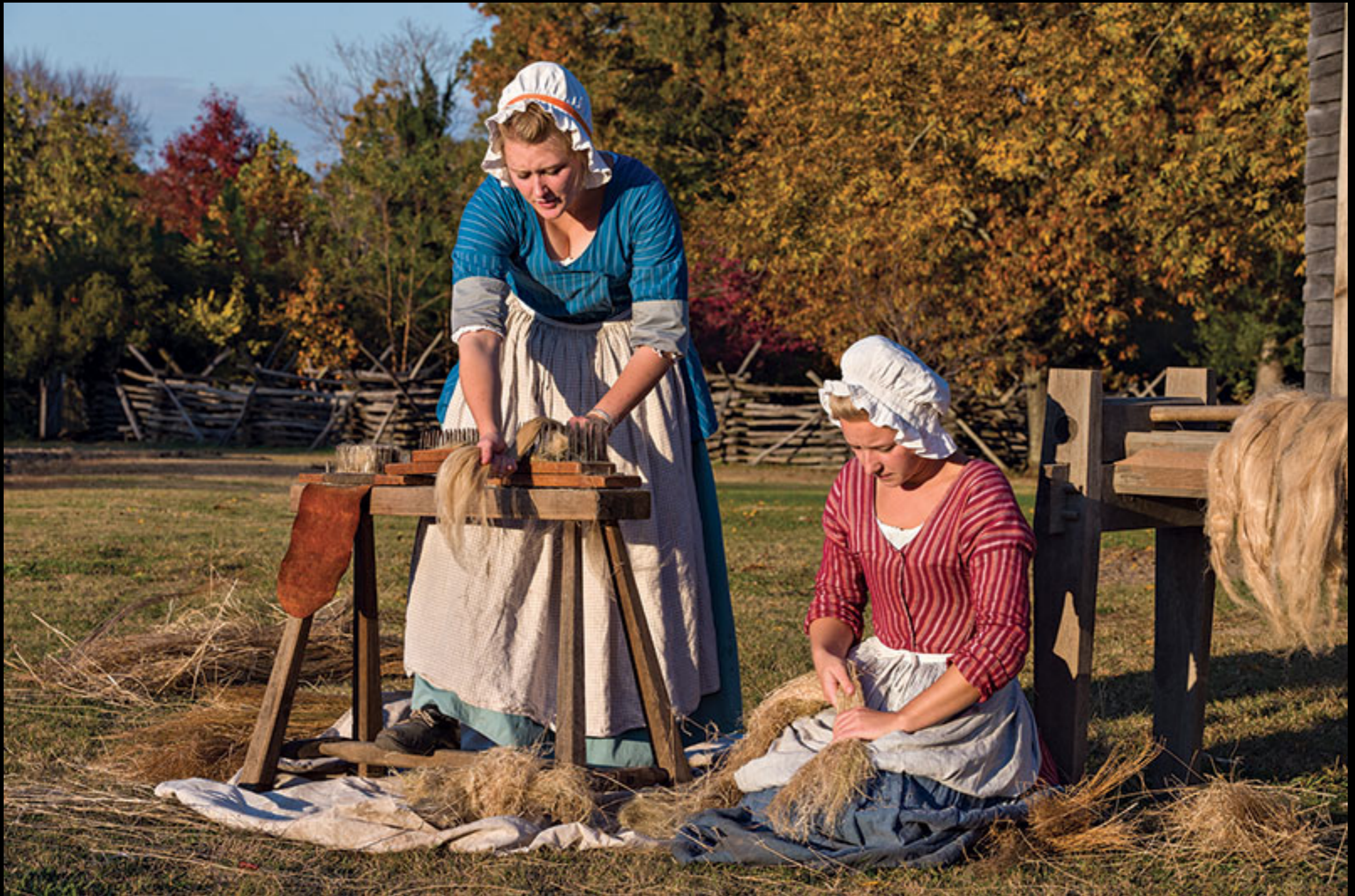
Flax Processing - Splitting and Straightening the Flax Fibers with a Heckle (Colonial Williamsburg Foundation - Dave Dooly Photograph - From "Flax & Hemp in Colonial America" by Ben Swenson)
