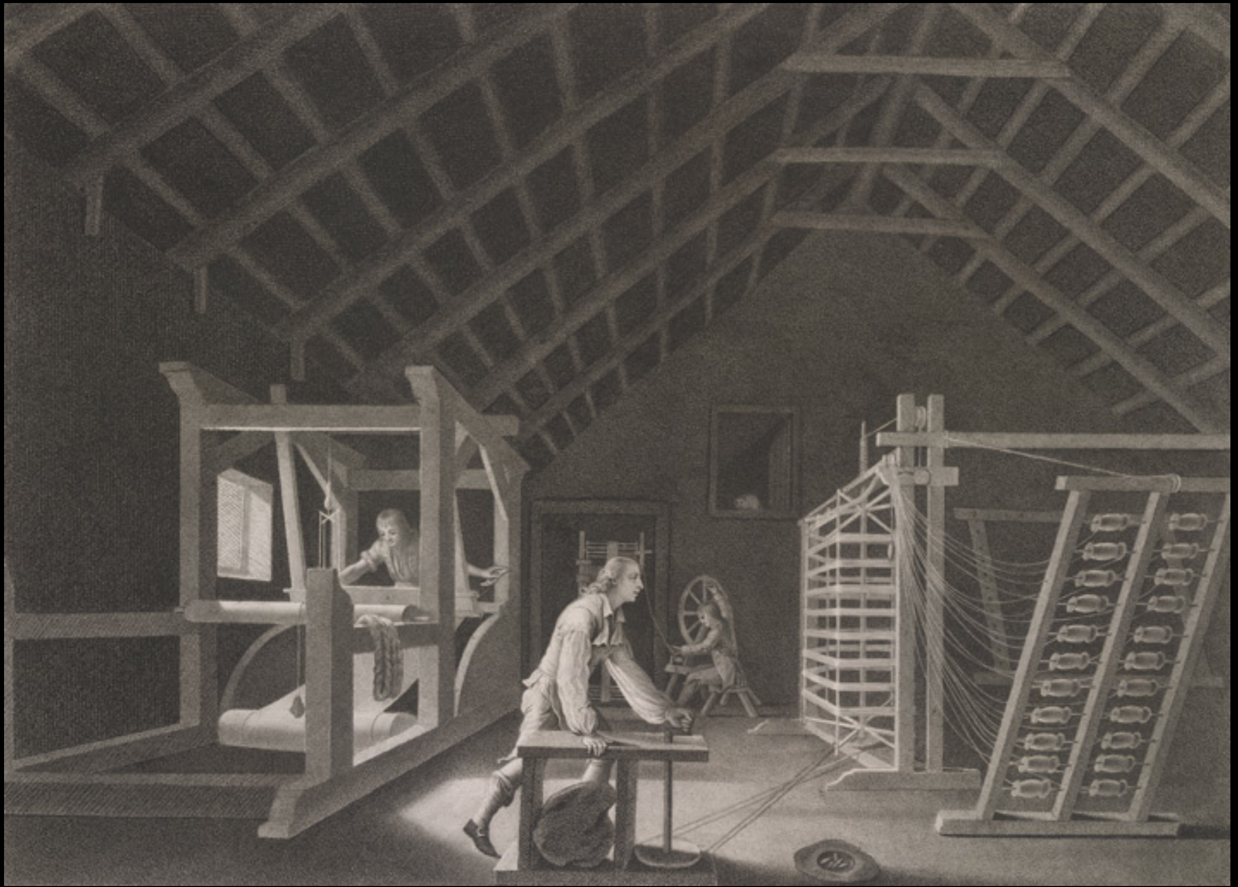
“Plate representing Winding, Warping with a new improved Warping Mill and Weaving” by William Hincks 1783 (The British Library)
