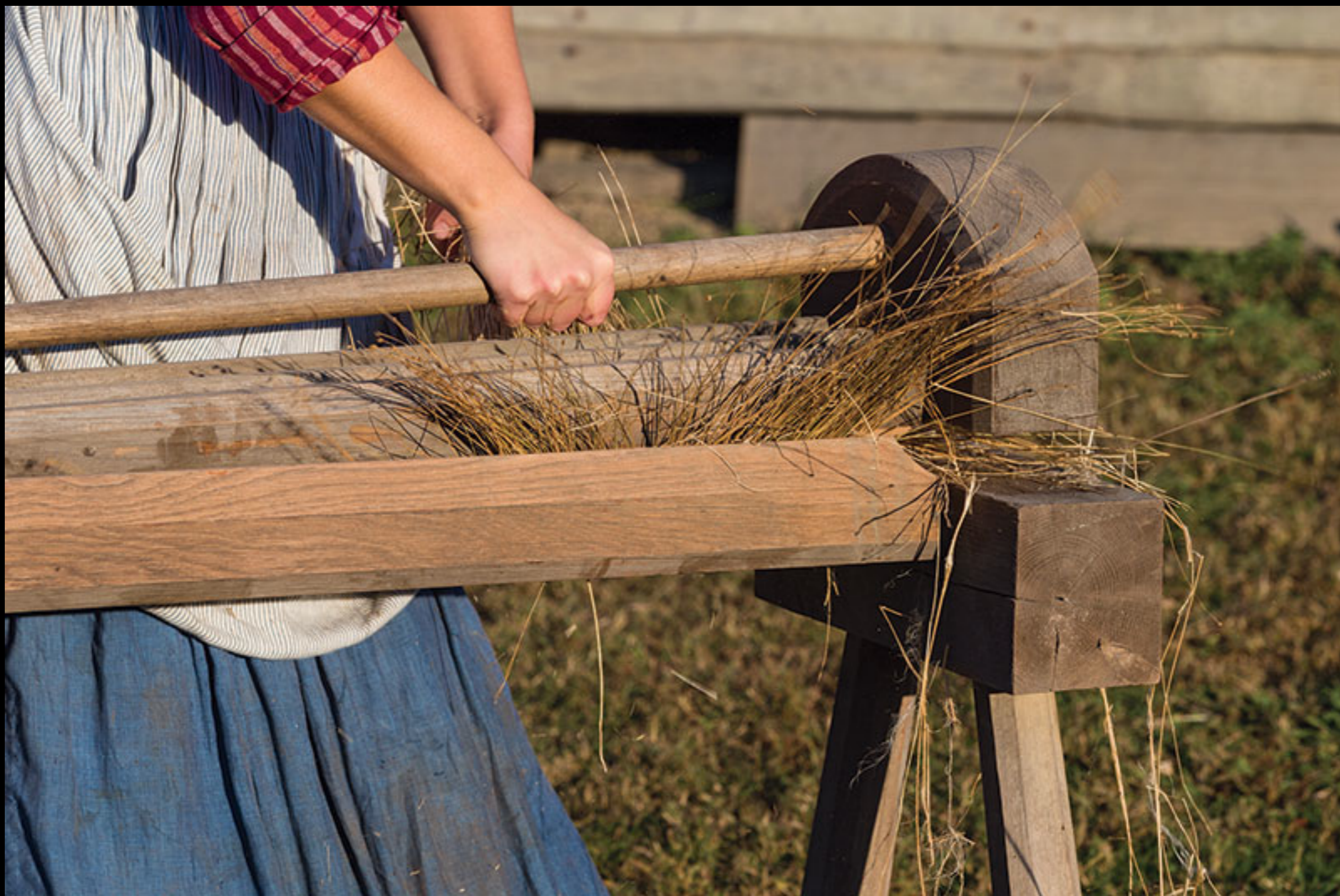
Flax Production - Using a Flax Break to Crush the Straw which Separates the Fiber from the Bark (Colonial Williamsburg Foundation - Dave Dooly Photograph - From "Flax & Hemp in Colonial America" by Ben Swenson)
