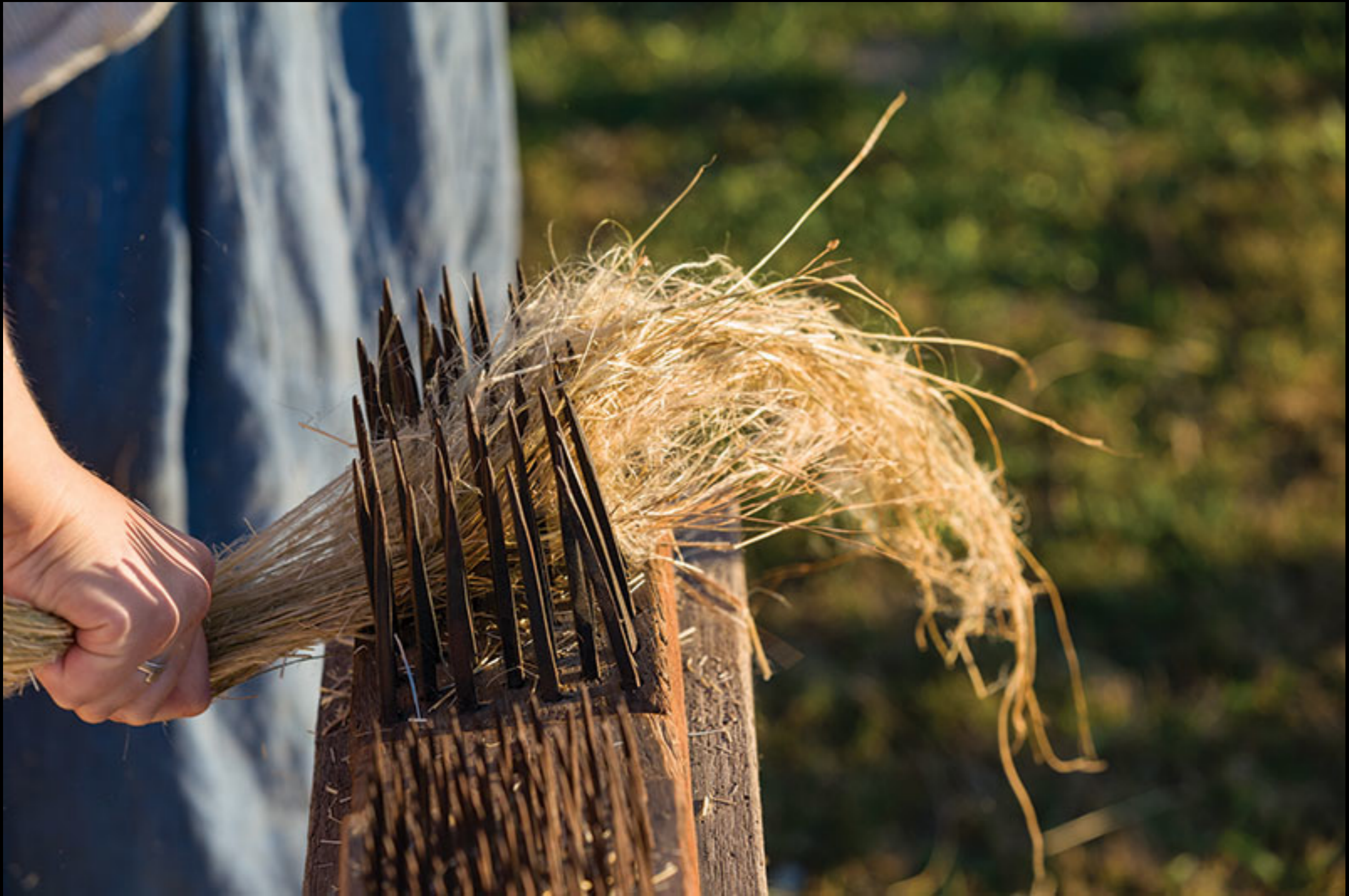
Flax Processing - Refining the Flax Fibers by Pulling them through the Iron Combs of a Heckle (Colonial Williamsburg Foundation - Dave Dooly Photograph - From "Flax & Hemp in Colonial America" by Ben Swenson)
