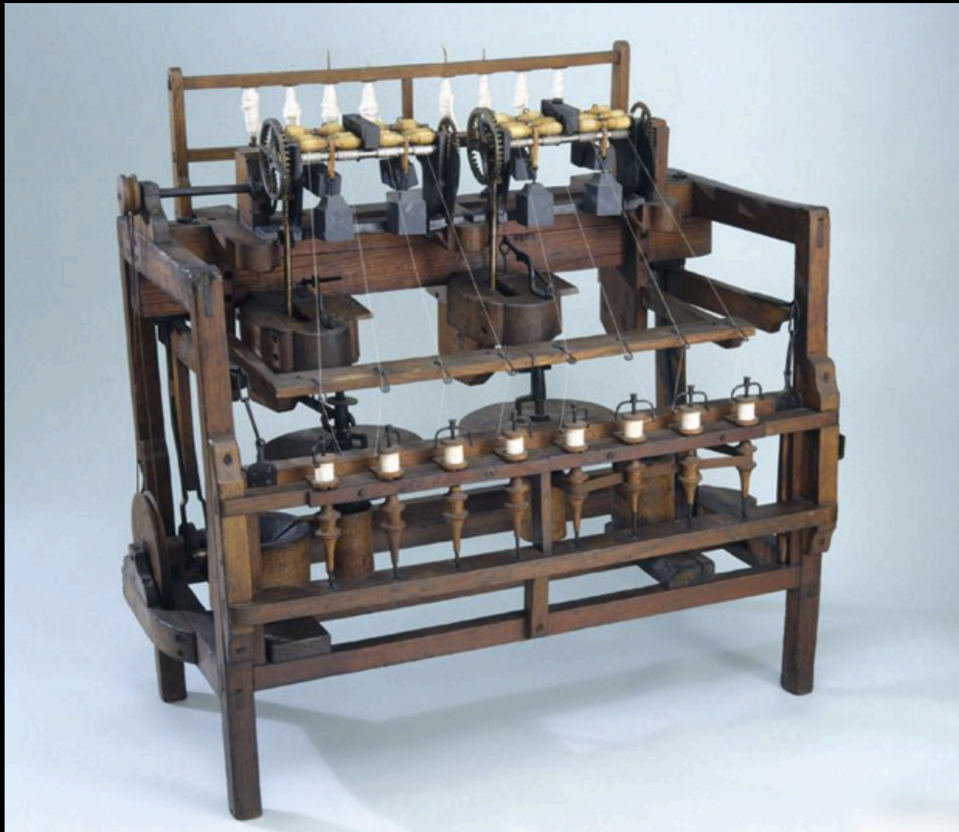
Sir Richard Arkwright's Improved Water Frame for Spinning Cotton Used at Arkwright's Cromford Mill at Matlock Bath in Derbyshire - Driven by Water 1775 (SCM)
