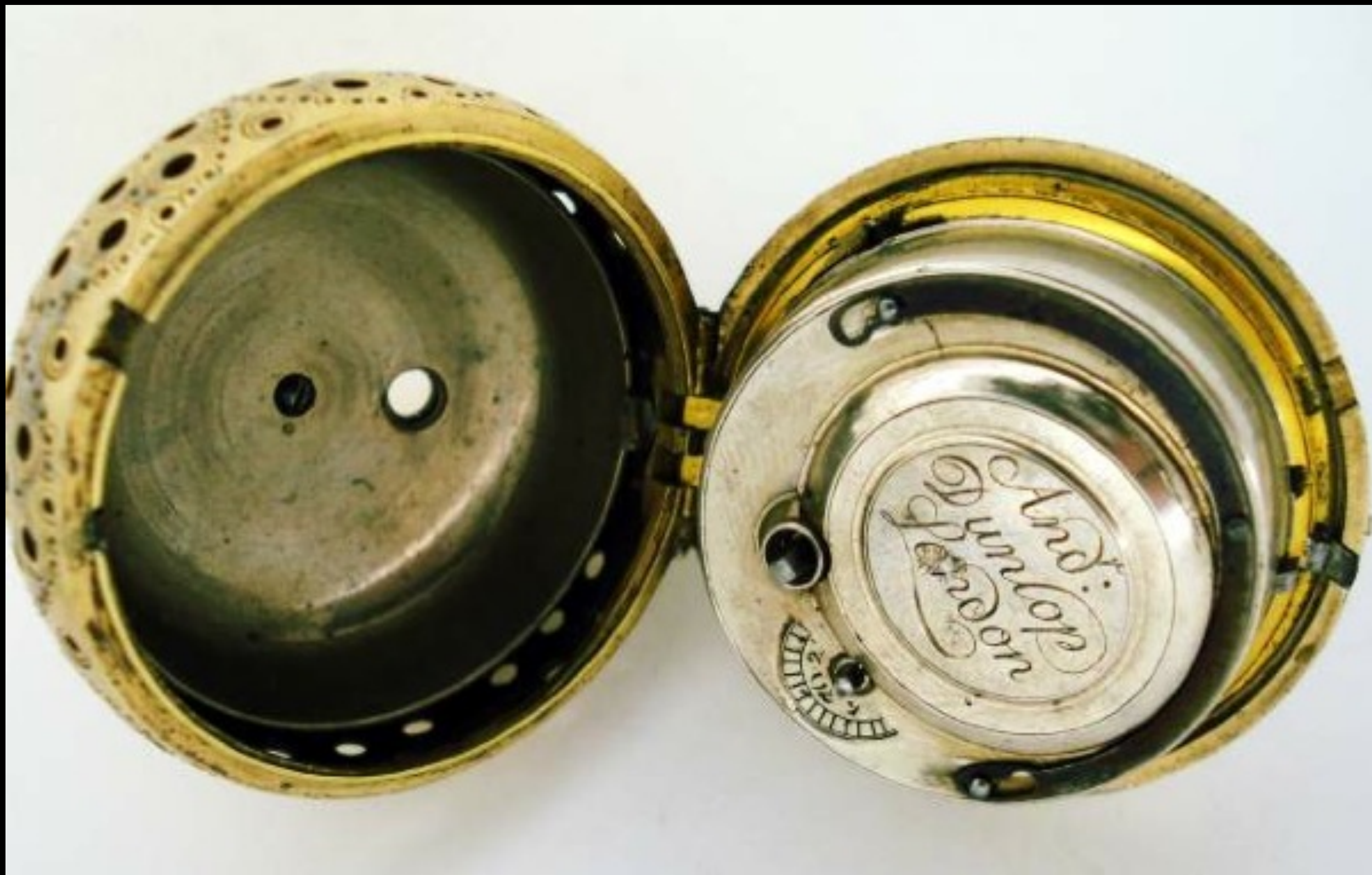
English Gilt Pair Cased Watch with Verge Movement, Quarter Repeat by Andrew Dunlop of London c. 1720 (Cogs & Pieces, Antique Pocket Watches)
