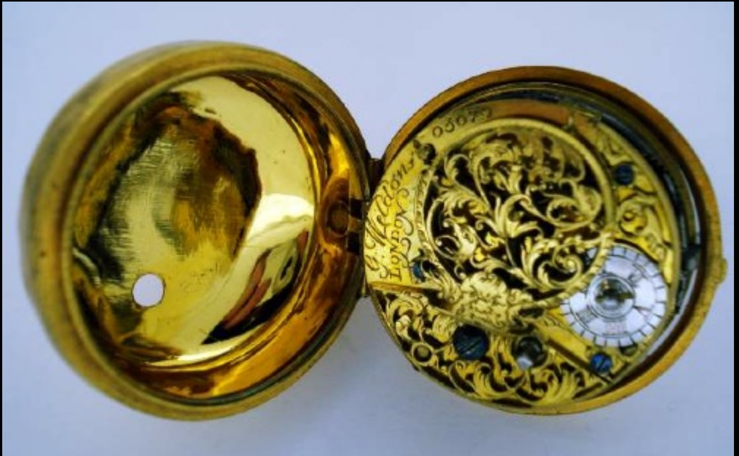
English Gilt Pair Cased Watch with Verge Movement by G. Weldon of London 1728 (Cogs & Pieces, Antique Pocket Watches)
