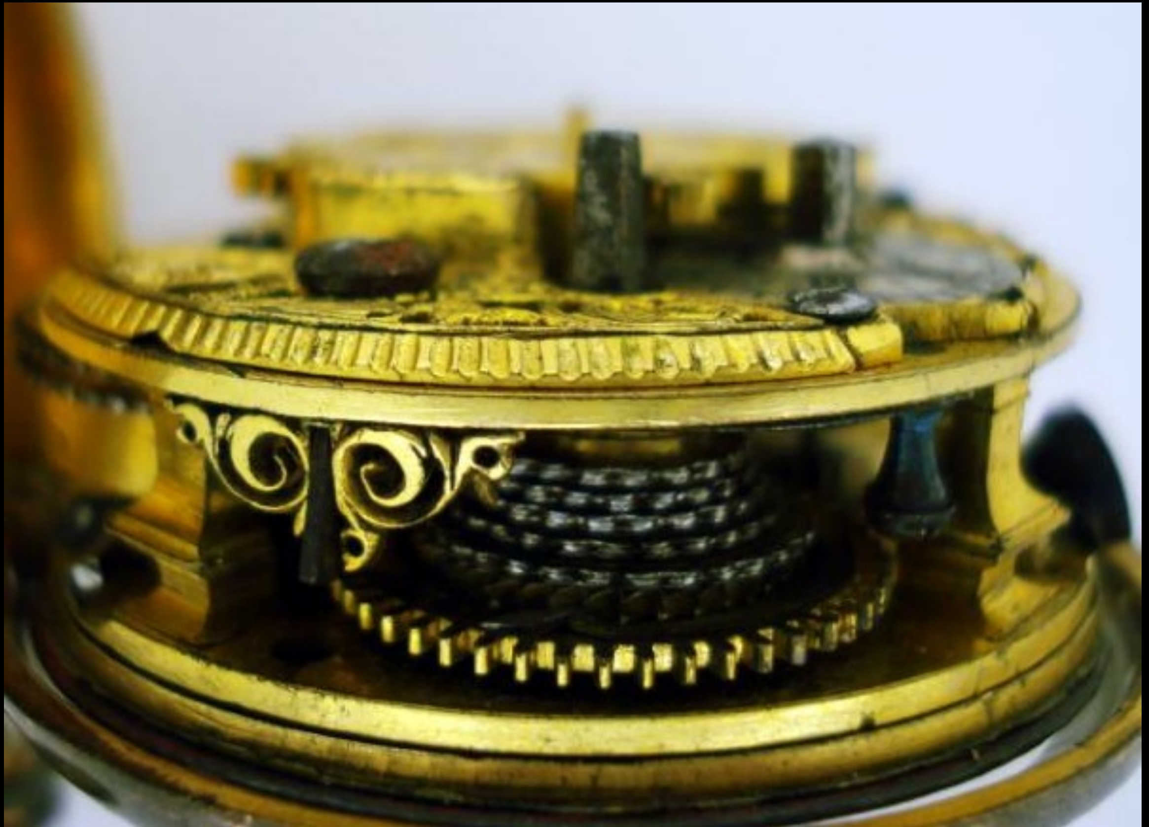
English Gilt Pair Cased Watch with Verge Movement by Henry Fish of London c. 1740 (Cogs & Pieces, Antique Pocket Watches)
