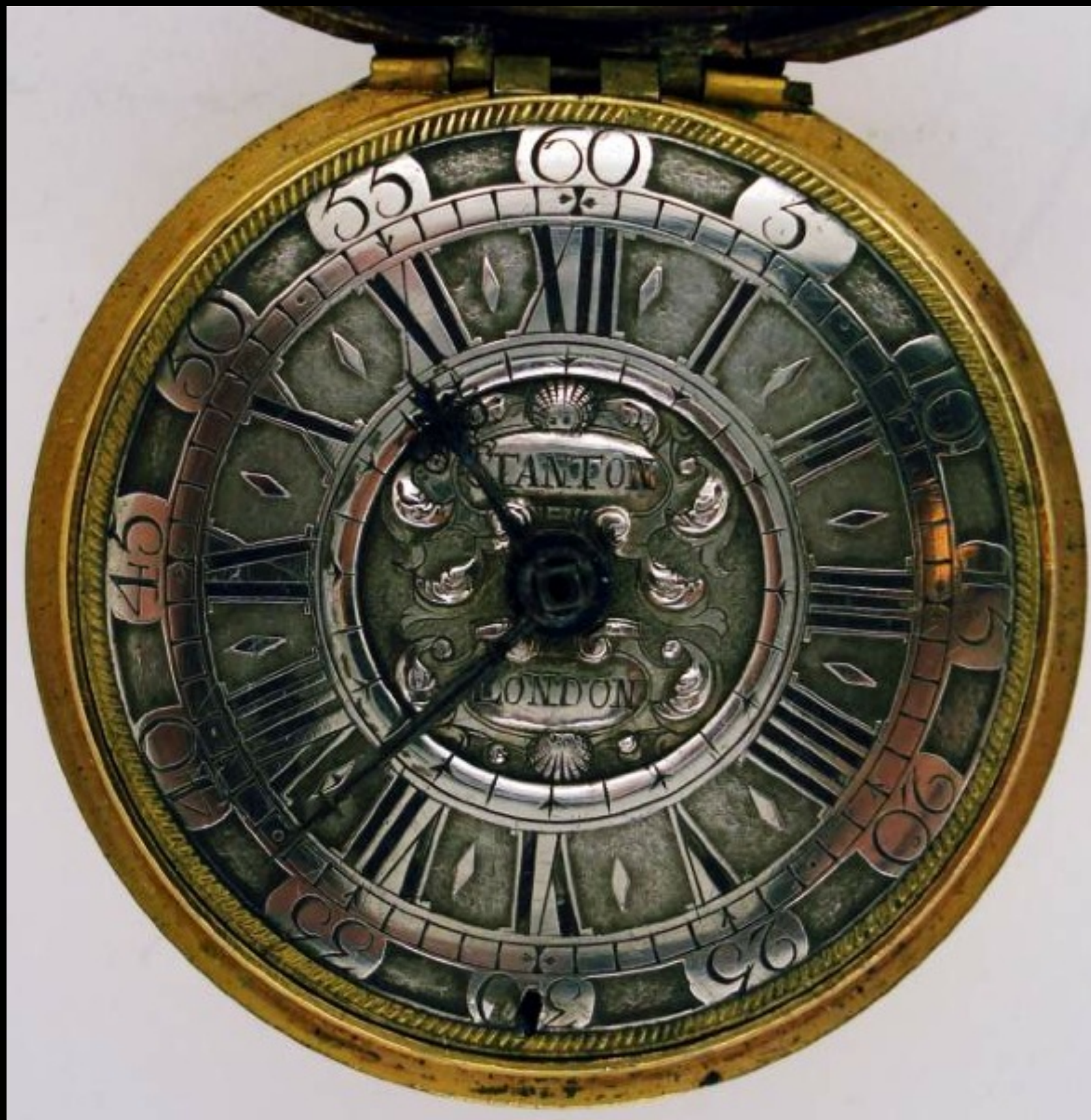
English Gilt & Shagreen Pair Cased Watch with Verge Movement by Edward Stanton of London c. 1680 (Cogs & Pieces, Antique Pocket Watches)
