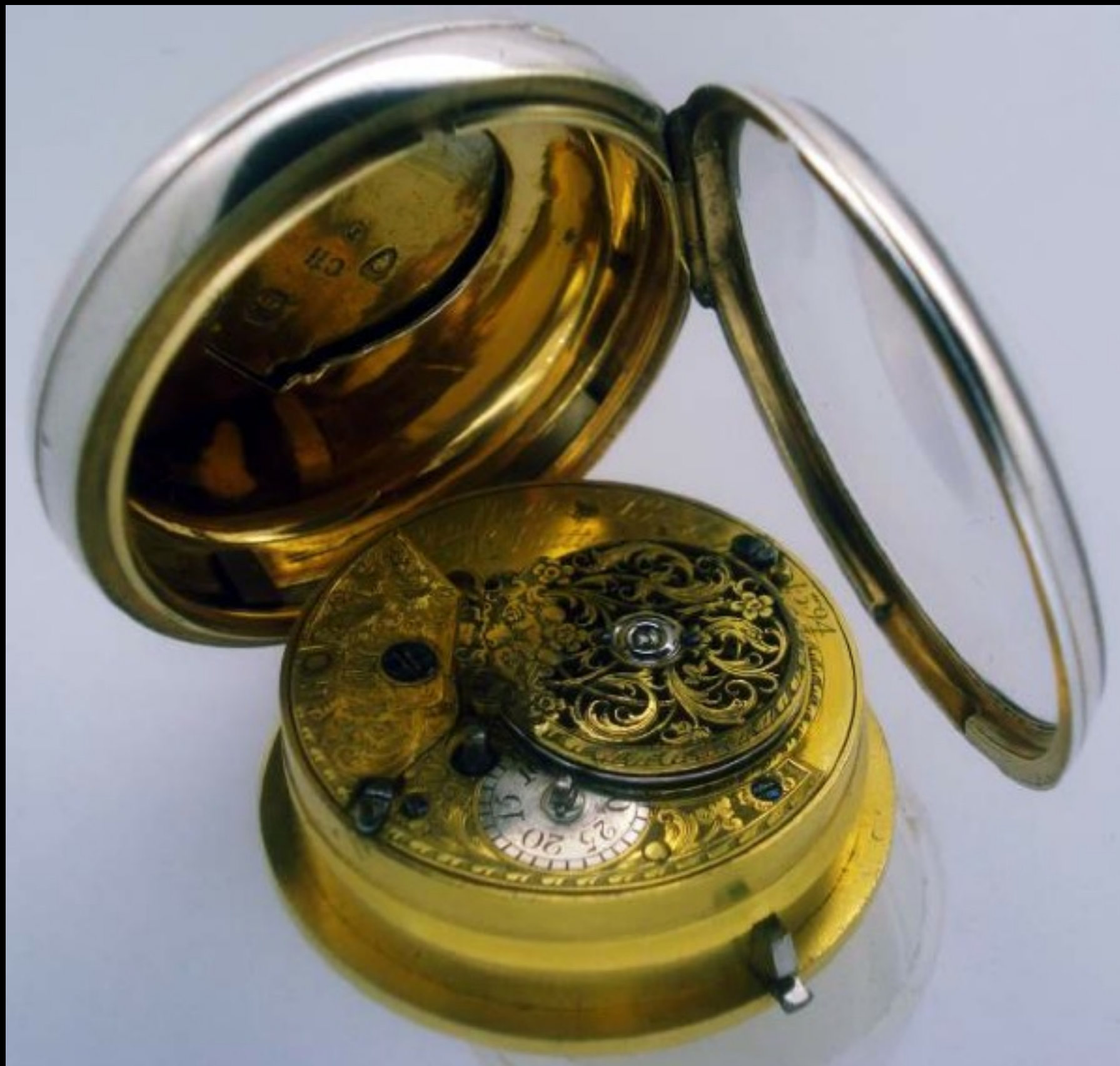
English Silver Pair Cased Watch with Cylinder Movement by Mudge & Dutton of London 1780 (Cogs & Pieces, Antique Pocket Watches)
