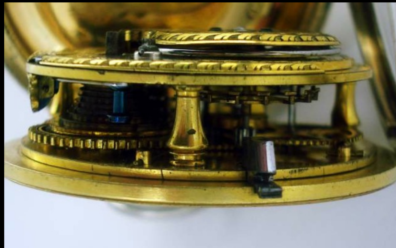
English Silver Pair Cased Watch with Cylinder Movement by Mudge & Dutton of London 1780 (Cogs & Pieces, Antique Pocket Watches)
