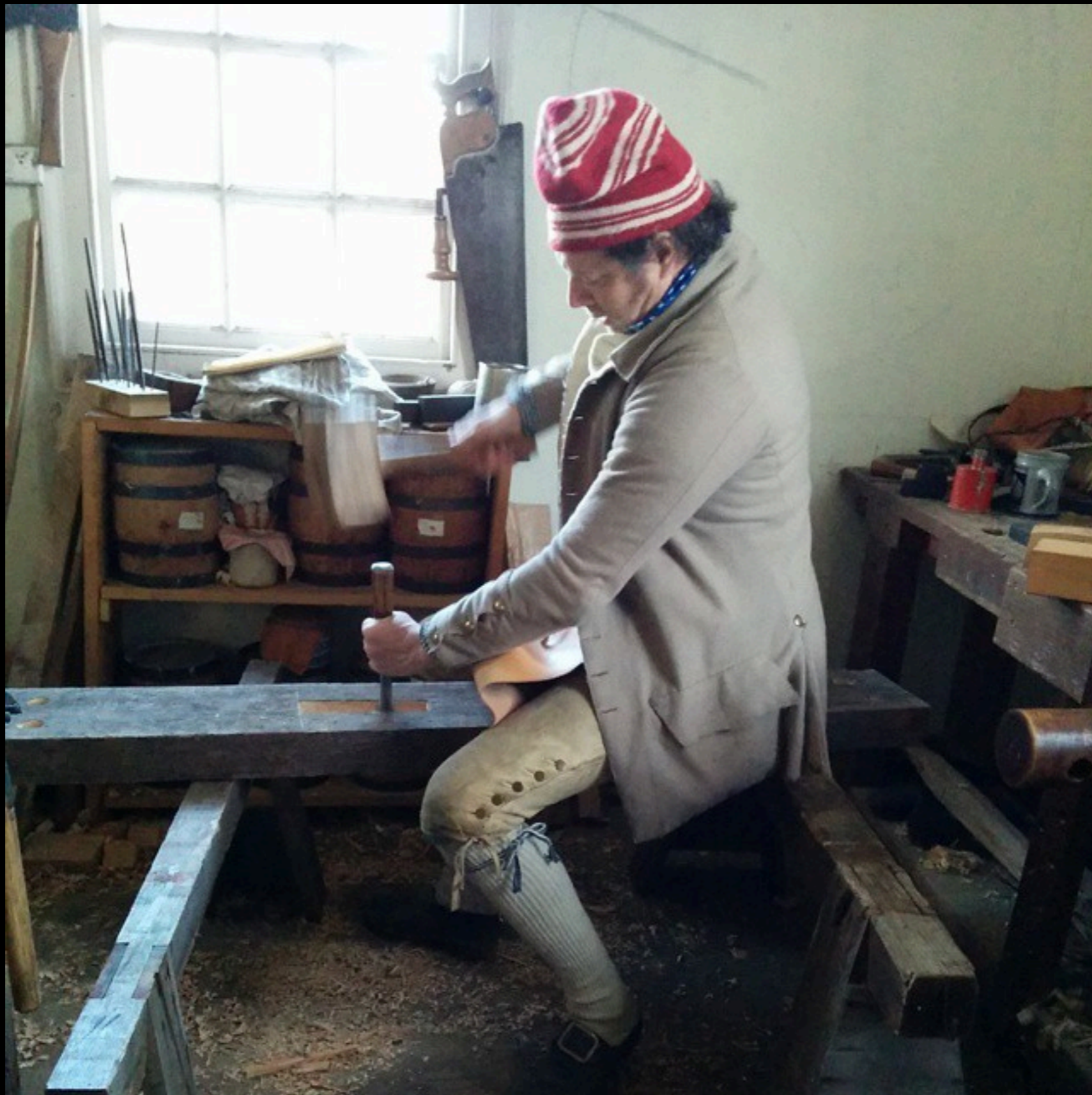
Working a Mortise at the Wheelright's Shop (The Wheelright's Shop at Colonial Williamsburg, Dana Shoaf - Photo Courtesy Heidi Campbell - Shoaf)
