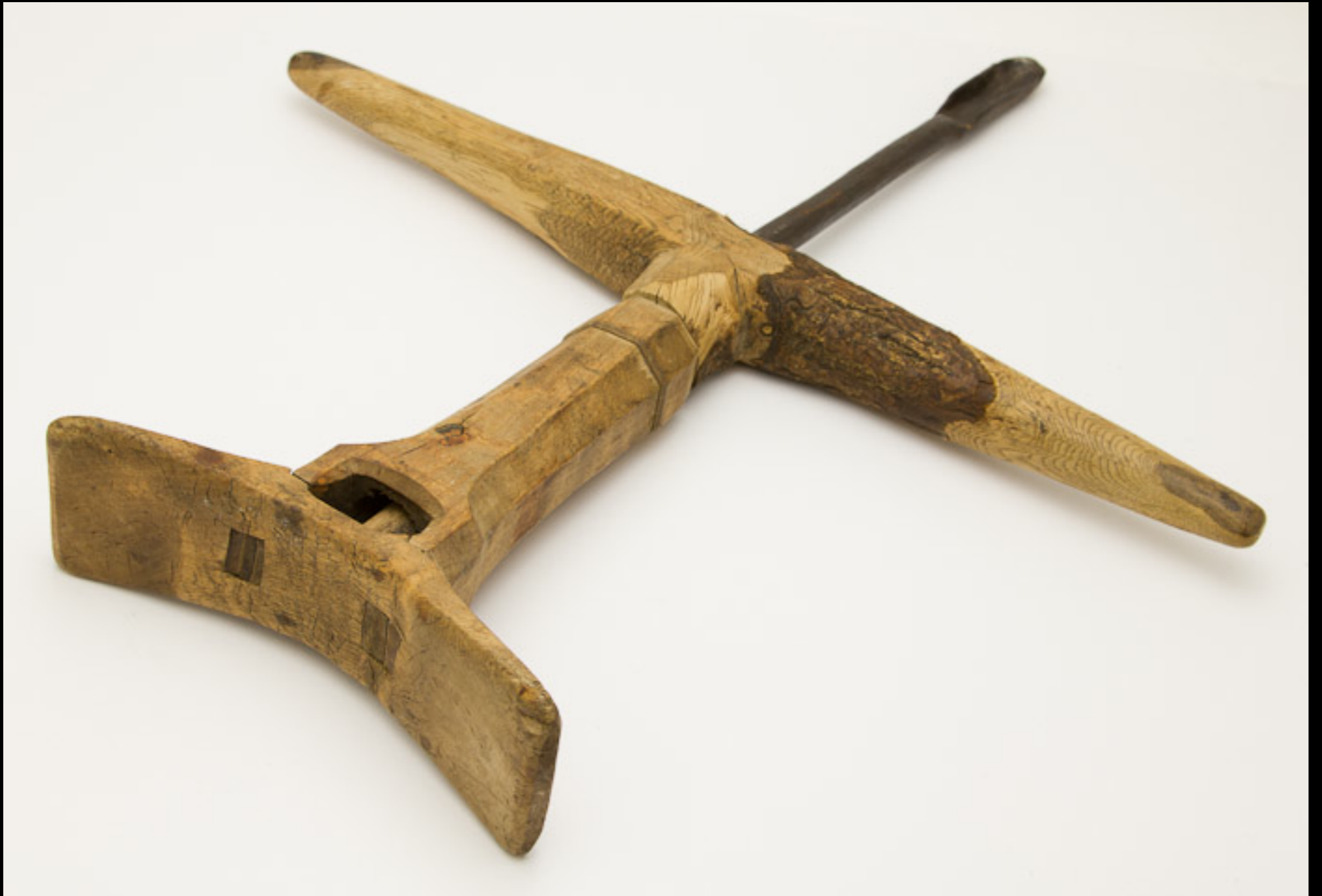
Chairmaker's Chest Brace with Spoon Bit 18th - Possibly Early 19th Century (Jim Bode Antique Tools)
