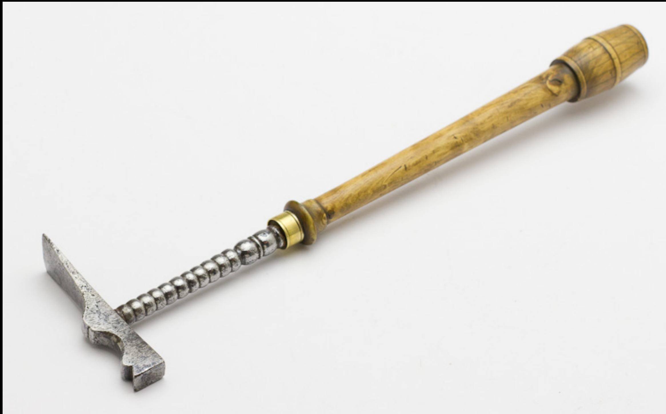
Tack or Upholster's Hammer with Boxwood Handle 18th Century (Jim Bode Antique Tools)
