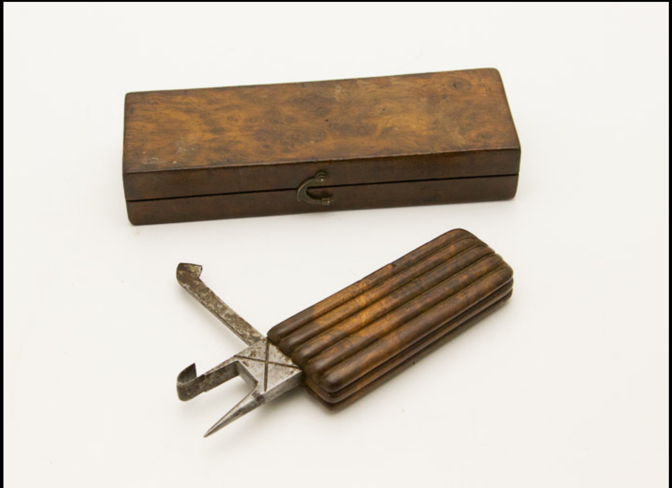
Burlwood Race Knife in a Burlwood Case 18th Century (Jim Bode Antique Tools)
