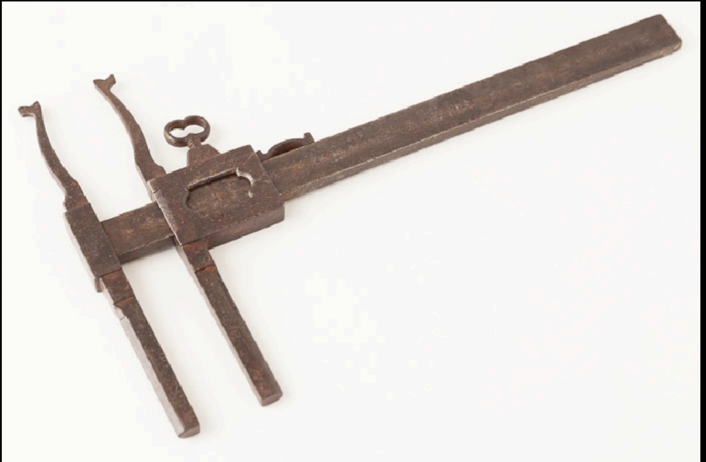
French Vernier Calipers by J. ROST 18th Century (Jim Bode Antique Tools)
