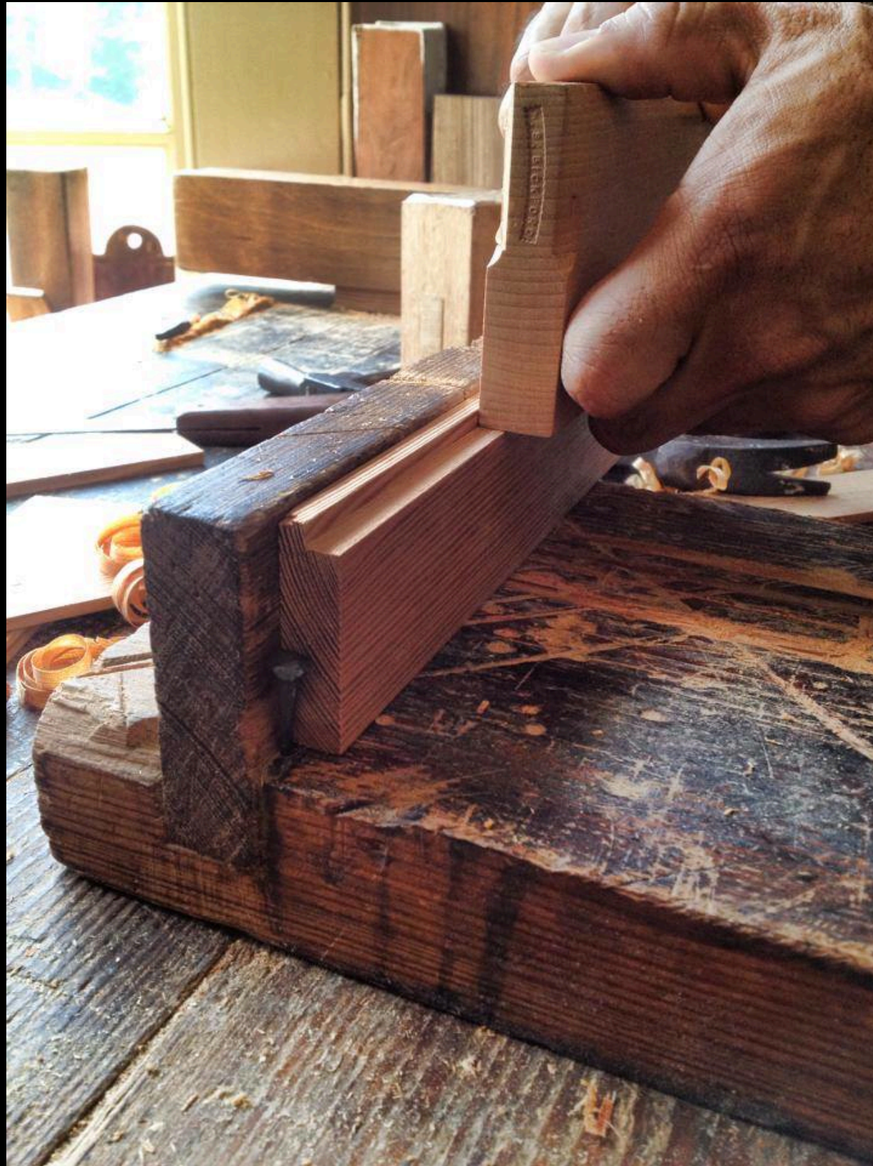
Improvised Shooting / Sticking Board to Cut a Rabbet / Rebate (The Joiner's Shop at Colonial Williamsburg)
