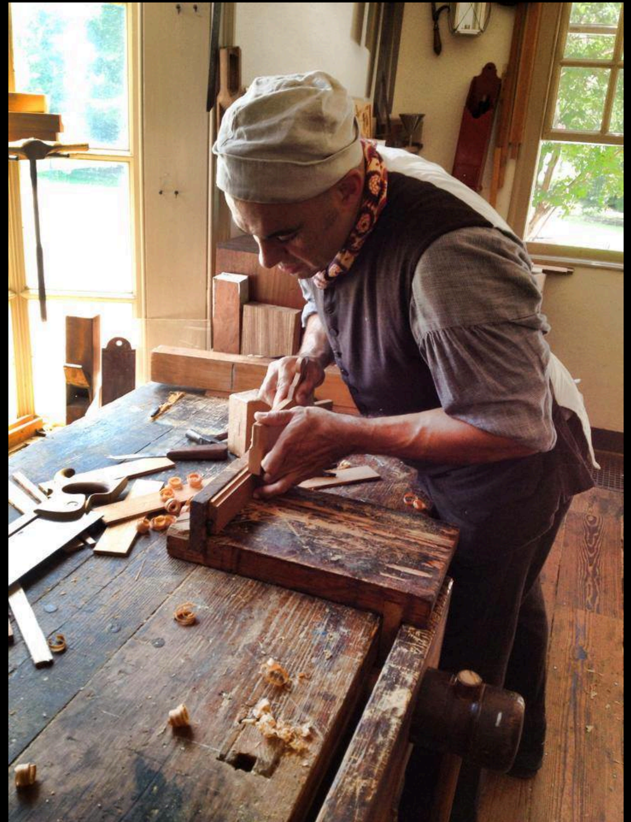
Improvised Shooting / Sticking Board to Cut a Rabbet / Rebate (The Joiner's Shop at Colonial Williamsburg)
