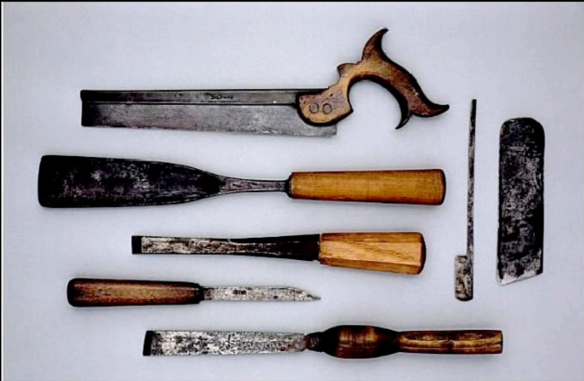
5. Eighteenth-century saw and edge tools made in Birmingham. Dovetail saw by Robert or William Dalaway; gouge, socket chisel (with new handle), and larger plane blade by Robert Moore; molding plane blade, probably by Aron Hildick (thought to be a Birmingham maker); mortise chisel by John Allen; and turning chisel by Sampson Freeth. Dovetail saw OL: 15". 1990-100; courtesy of the Framingham Historical and Natural History Society, Framingham, Mass.; 1984-184; courtesy of Martyl and Emil Pollak; courtesy of the Paul B. Keabian Collection; 1990-236; 1992-199.
