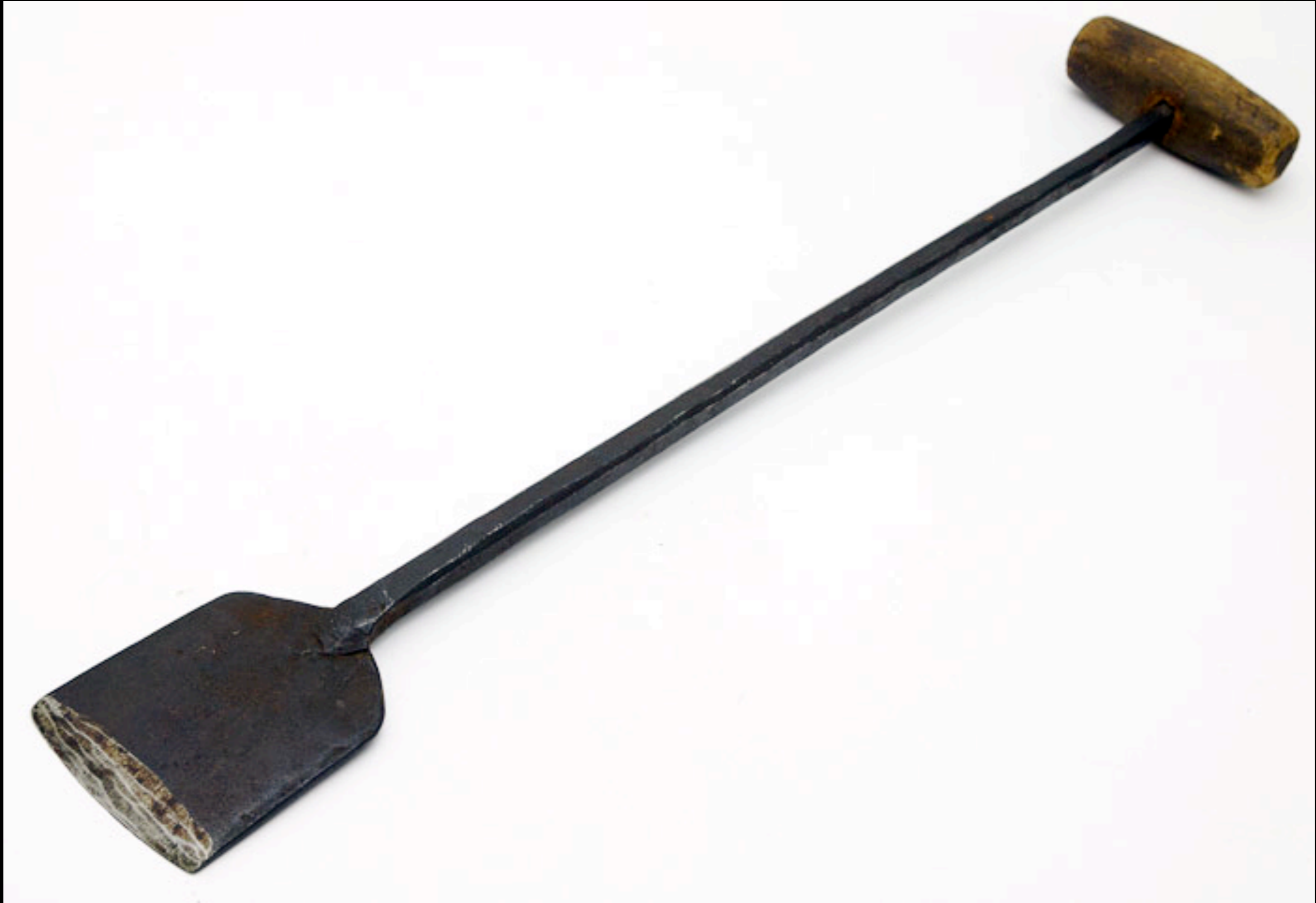
Bark Spud for Removing Bark 18th Century (Jim Bode Antique Tools)
