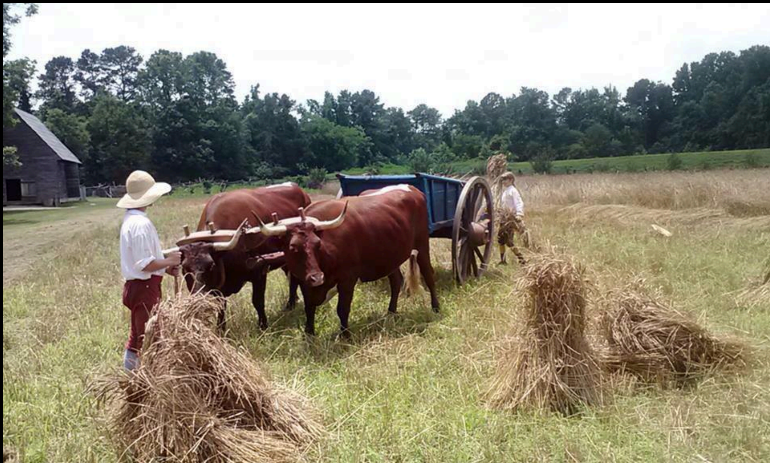
Ox Cart Recreated from Plantation Owner, Landon Carter's, Diary Capacity of 40 Bushels or 1.5 Tons of Manure (Historic Carpenters of Williamsburg - Fabricated by the Deane Shop)
